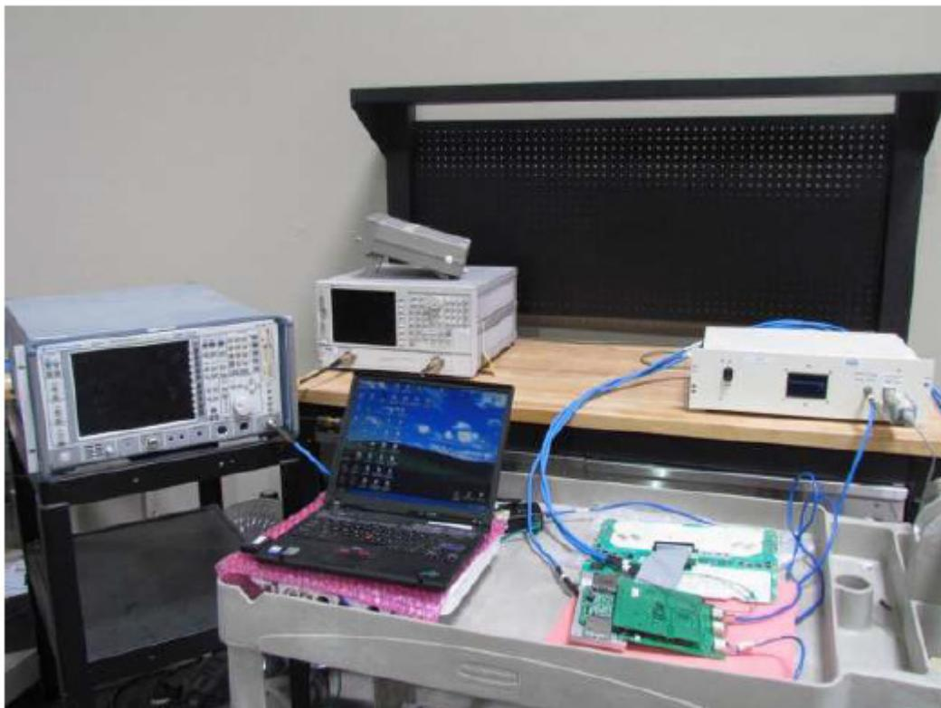
**6.2. Test Setup - Digital Emissions <1 GHz**
