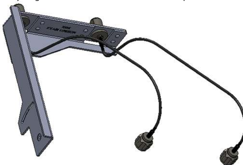
Figure 10. Attaching Antenna Cables to L-Bracket
