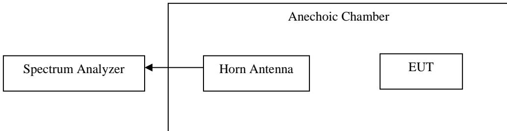
This setup is used for measuring the radiated output power in a fully anechoic chamber with a measurement distance of 1m.
