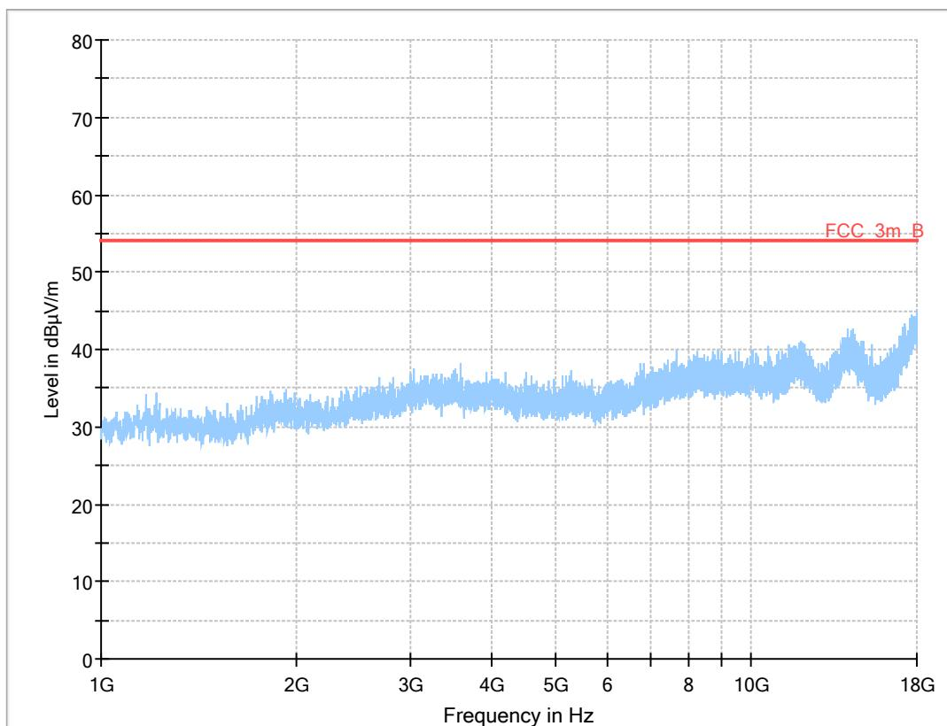
**The radiated spurious emission of the unintentional radiator is below the indicated limit.**
