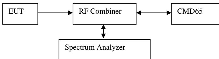
This setup is used for all conducted emission tests.
