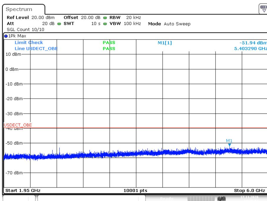
Out-of-Band Unwanted Emissions, Conducted,  $\Pi/4$ -DQPSK
