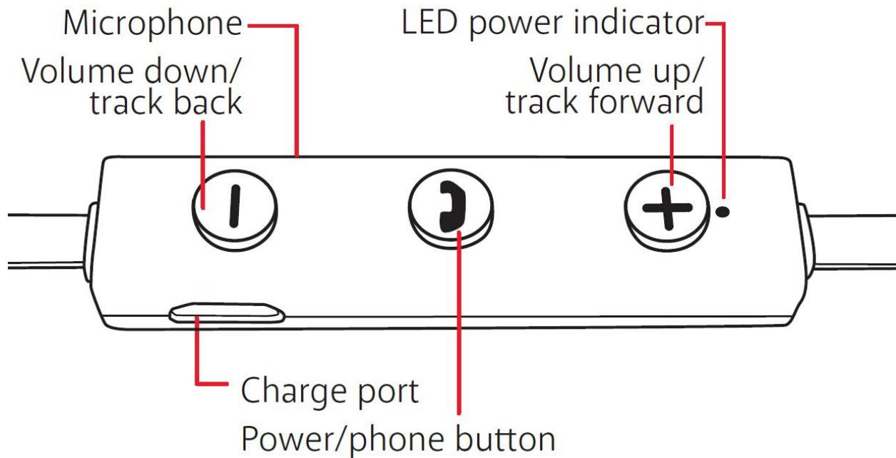
(volume up/track forward button, power/phone button, volume down/track back button), the power LED indicator light next to the plus button and the microphone under the control box]
