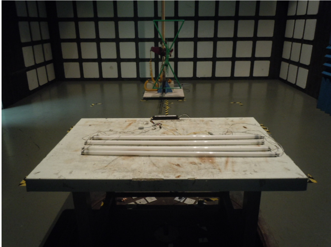
FRONT VIEW OF RADIATED EMISSION TEST
