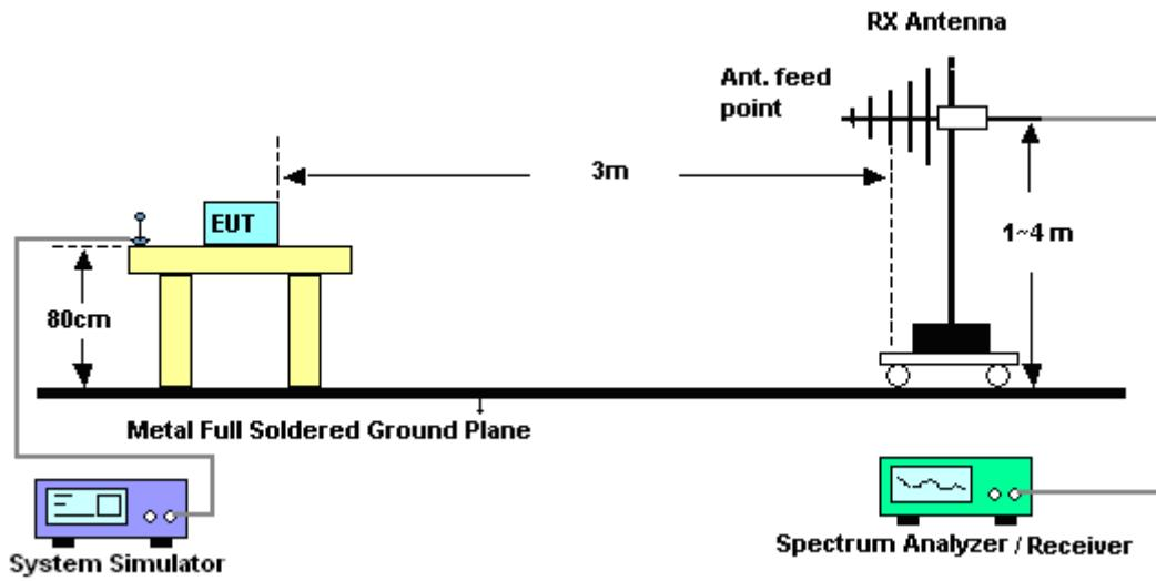
For radiated test above 1GHz
