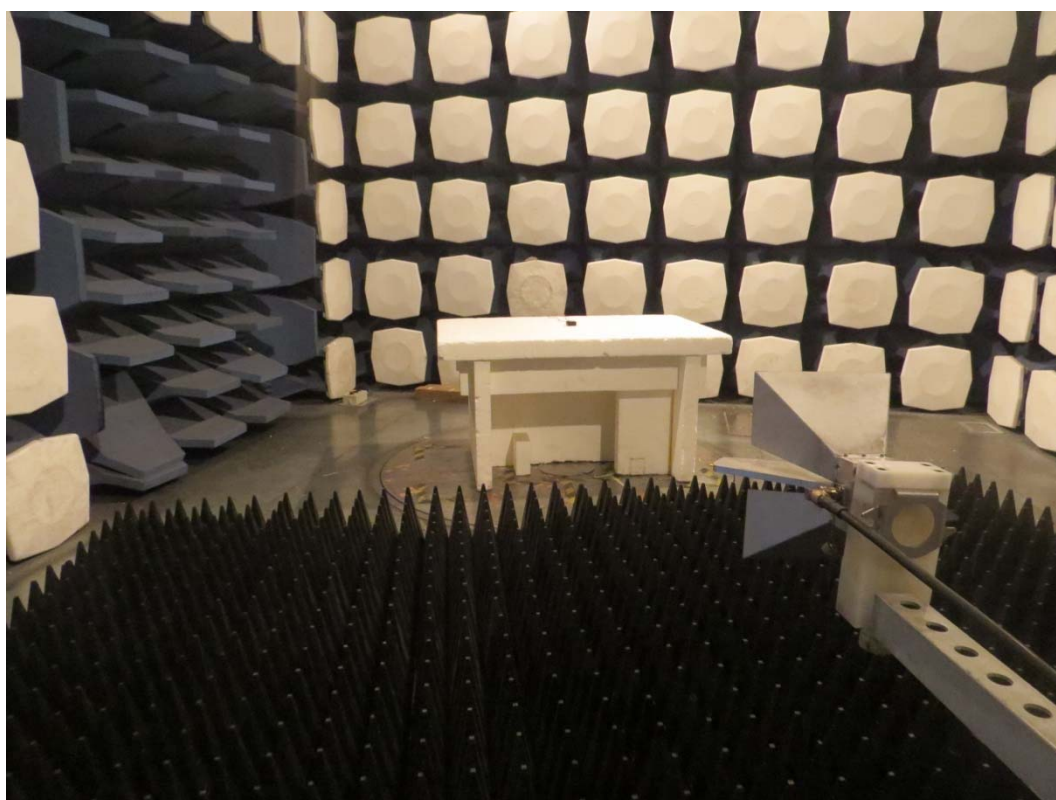
Picture 2: Radiated Spurious Emissions Test setup
