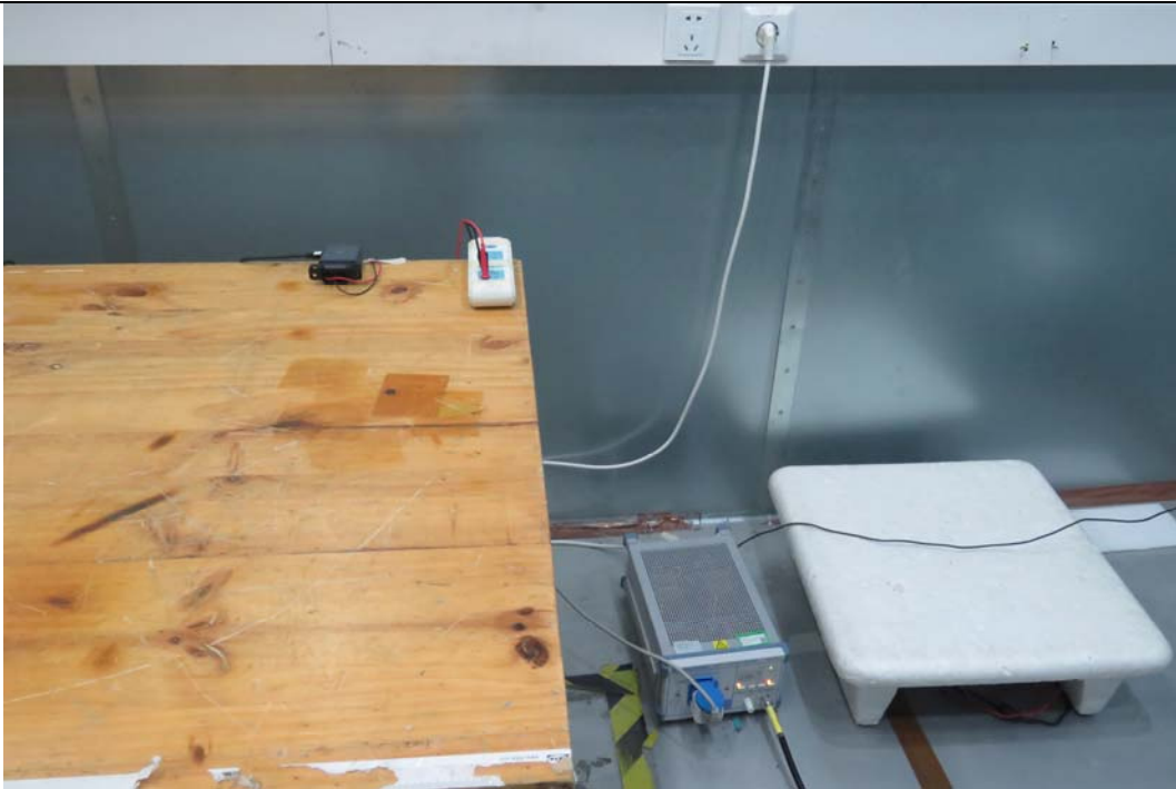
Picture 3 Conducted Emission Test Setup
