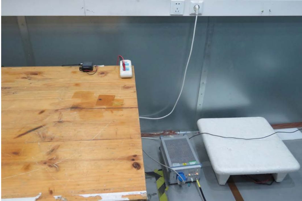
Picture 3 Conducted Emission Test Setup
