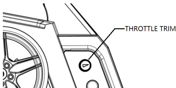
The TH-TRIM knob is used to adjust the throttle trim when the throttle stick is at neutral position. It is typically used to adjust the brakes.
