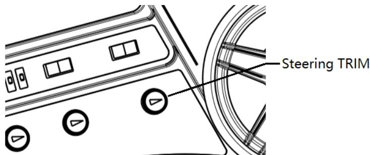
The ST-TRIM knob is used to adjust the trim of the steering so that the wheel is centered and the vehicle tracks straight.
