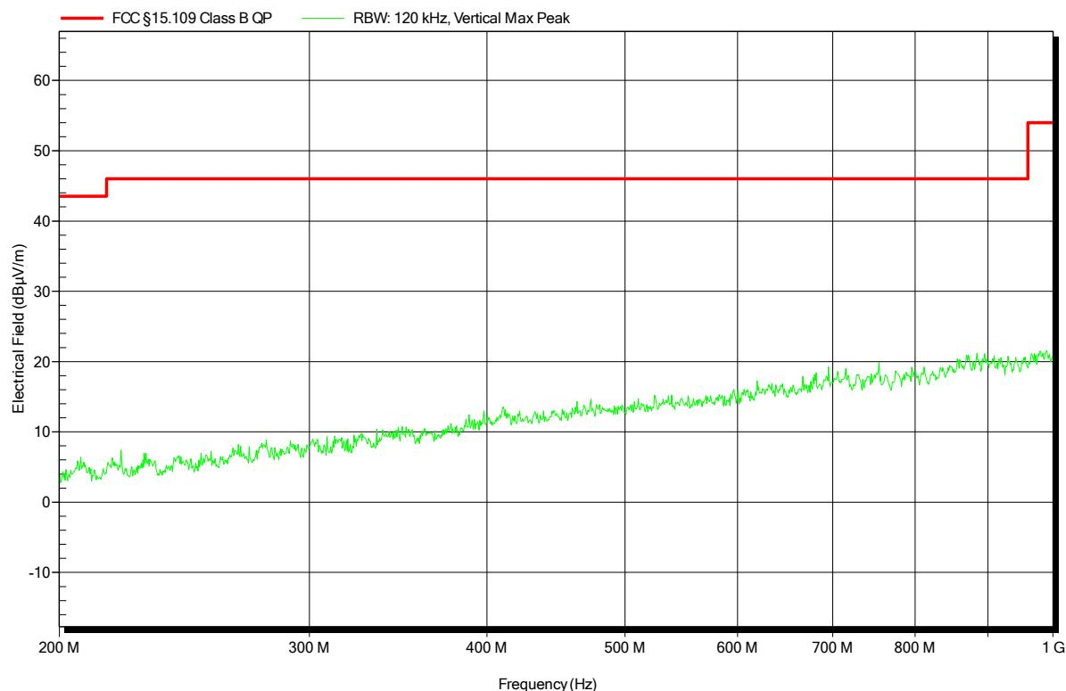
**Radiated emissions according to FCC 15B**
