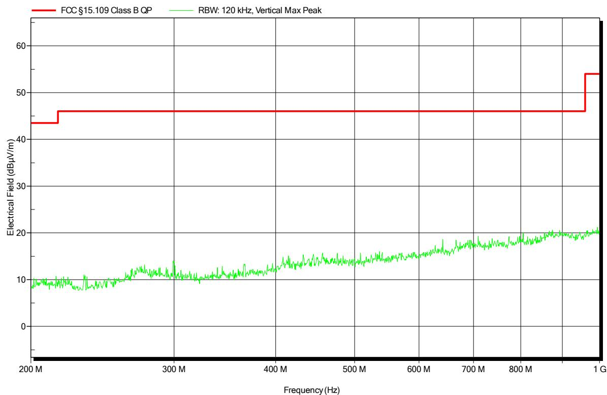
**Radiated emissions according to FCC 15B**
