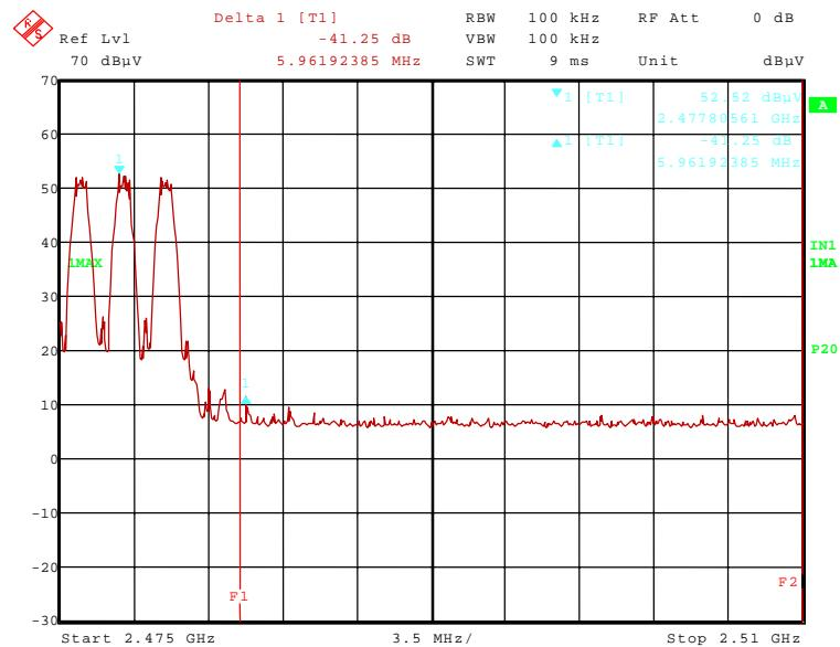
The plots on the pages before are showing the radiated band-edge compliance for the lower and upper band-edge. The frequency line 1 (F1) shows the upper and the frequency line 2 (F2) shows the lower edge of the assigned frequency band.
