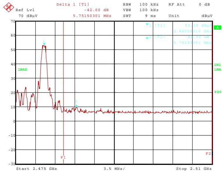
120795\_40.wmf: Radiated band-edge compliance, upper band edge, hopping on (operation mode 4):
