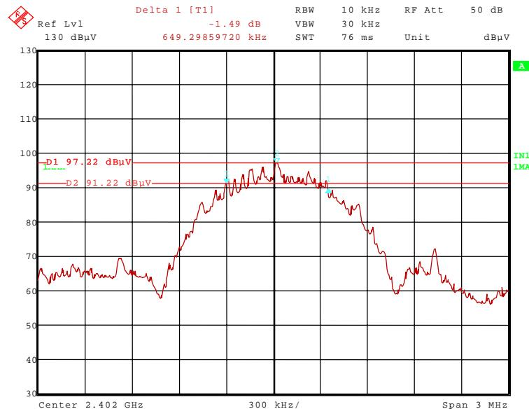
120795\_30.wmf: 6 dB bandwidth at the middle of the assigned frequency band (mode 2):
