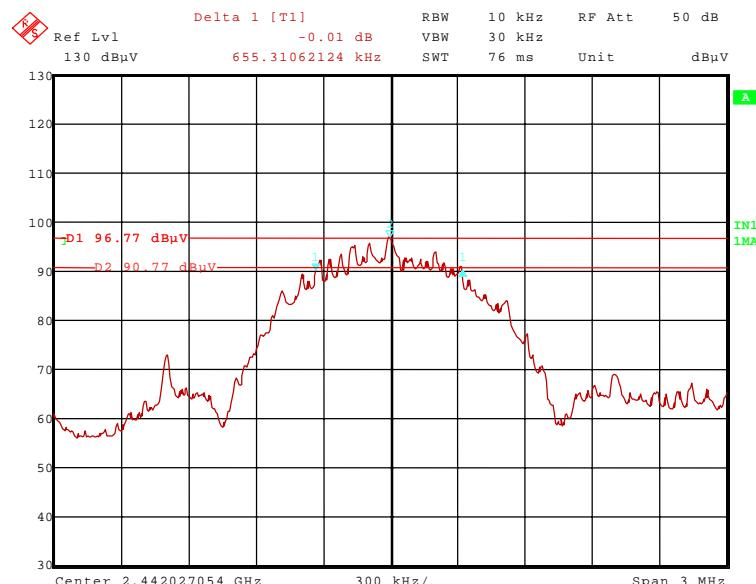
120795\_31.wmf: 6 dB bandwidth at the upper end of the assigned frequency band (mode 3):
