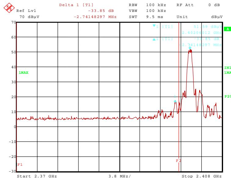
120795\_39.wmf: Radiated band-edge compliance, lower band edge, hopping on (operation mode 4):
