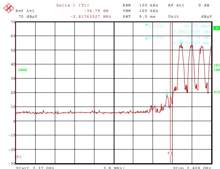
120795\_41.wmf: Radiated band-edge compliance, upper band edge, hopping off (operation mode 3):
