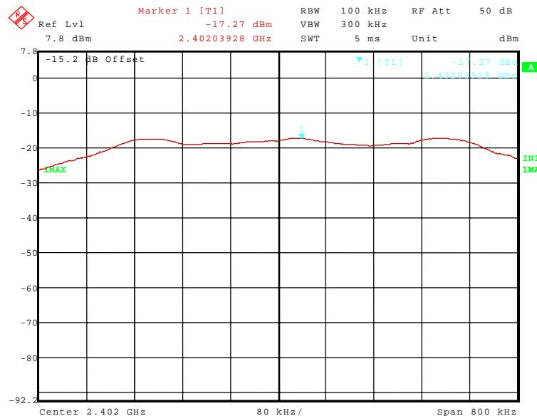
120795\_36.wmf: Power spectral density at the middle of the assigned frequency band (mode 2):
