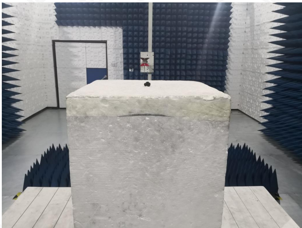
RADIATED EMISSION TEST SETUP ABOVE 1GHZ
