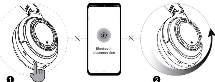
1. Manual power off: long press 5 seconds to power off, the red light will light up 3 times. The power off function is shielded during incoming call or in a call
