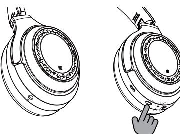
Turn off the headphone, long press the power button for 10 seconds, the red and blue lights 3 times, reset successful
