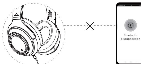
Once the audio cable is plugged in, the power will be cut off, the Bluetooth function will be disabled
