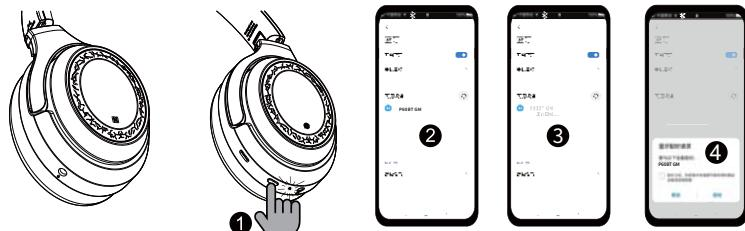
1. 3-click power button to automatically enter the pairing state, the red-blue light flashing quickly
