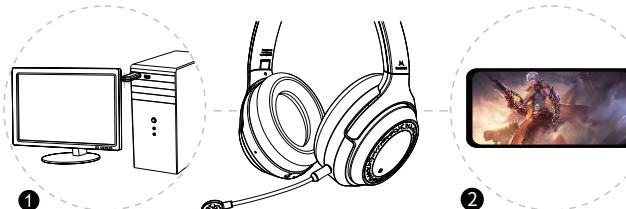
1. The headphone has been connected with the wireless transceiver at the factory. Turn on the headphone, plug the wireless transceiver into the computer, the headphone will connect automatically. If need to connect the phone with the headphone, please help to follow the instructions 8
