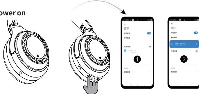
1. Long press the button for 3 seconds to turn on the headphone, it will automatically enter the pairing state when there is no connection. The red-blue indicator blinks, the voice prompts "Power on"
