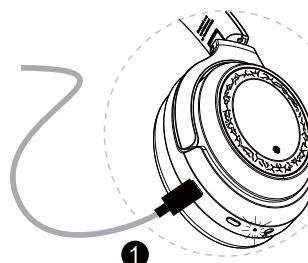
1. Being charged when the headphone is on: the red and blue lights will flash, and the blue light is on when fully charged
