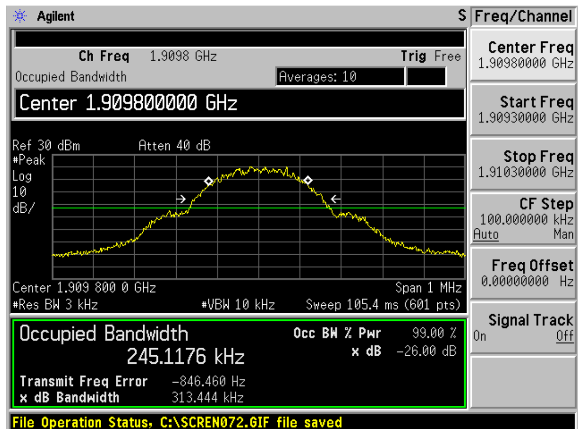
GSM 1900 GPRS CH810 Occupied Bandwidth
