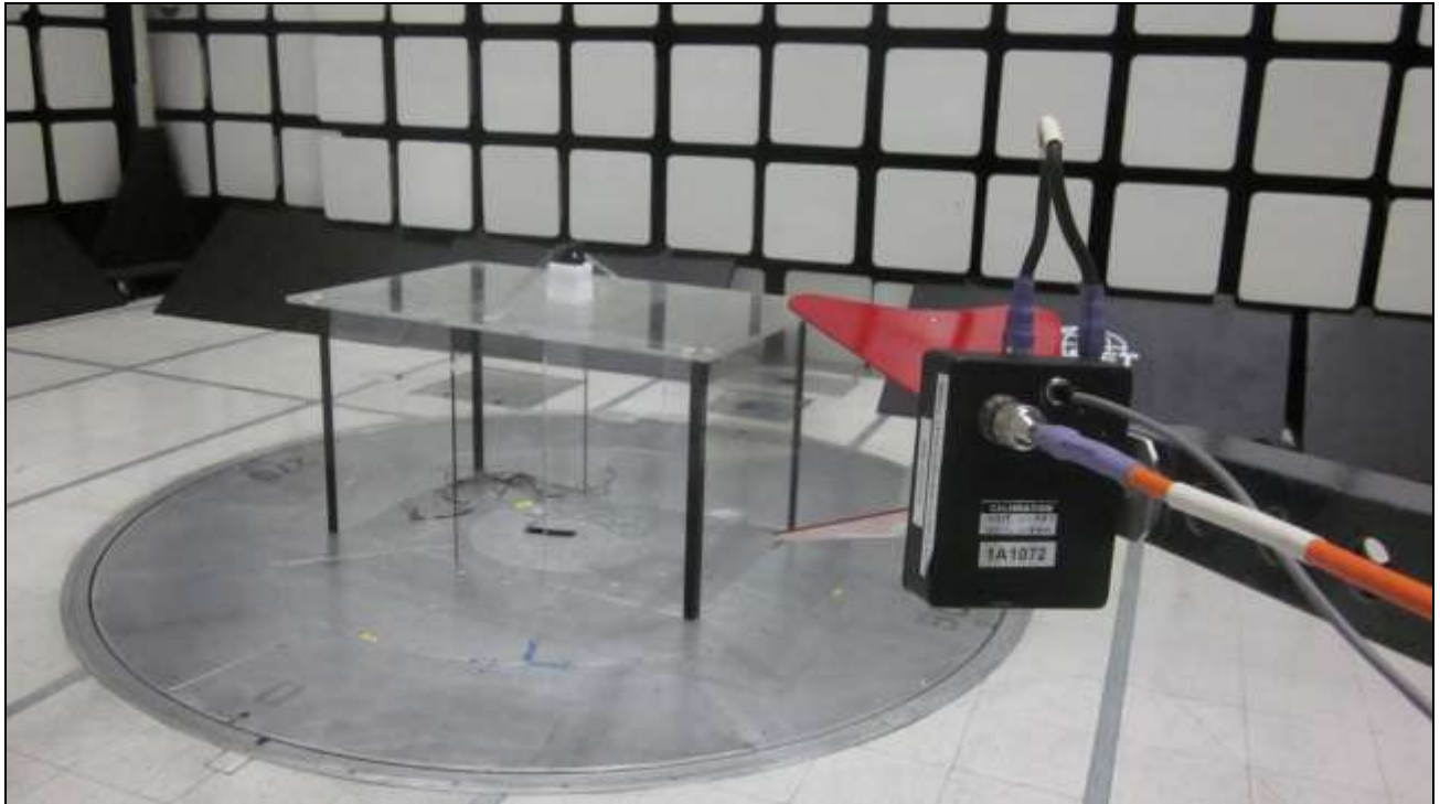
Photograph 7. Field Strength of Fundamental, Test Setup
