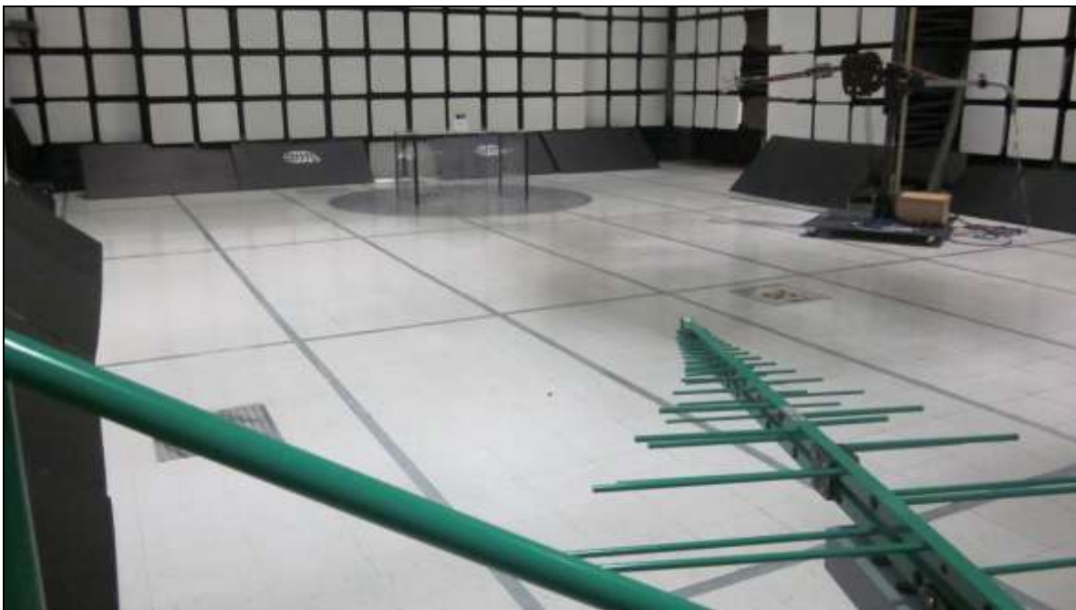
Photograph 8. Radiated Emissions, Test Setup, 30 MHz – 1 GHz
