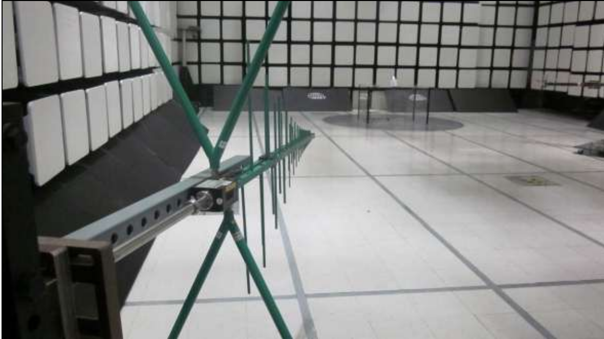
Photograph 5. Radiated Emissions, Test Setup
