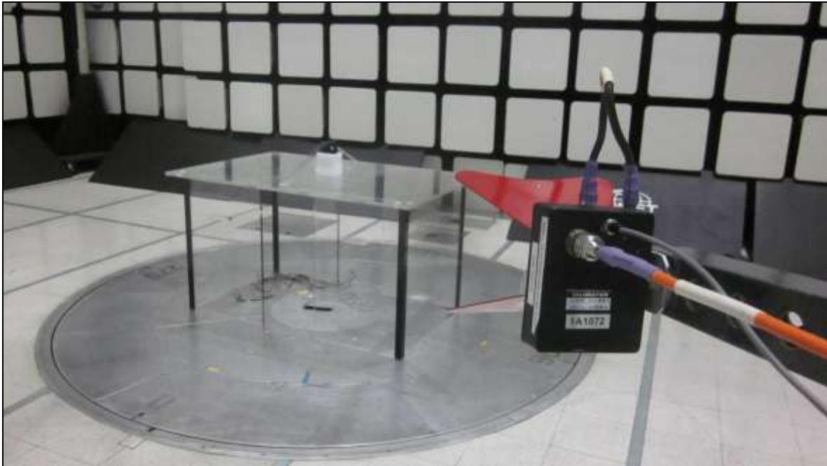
Photograph 9. Radiated Emissions, Test Setup, 1 GHz – 18 GHz
