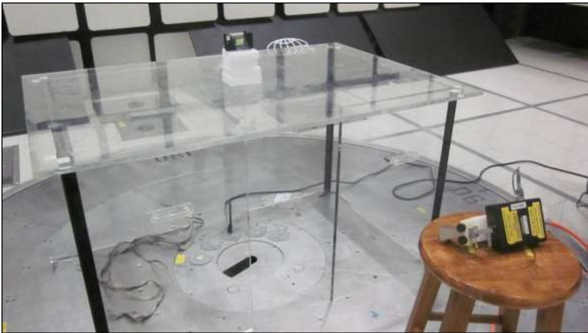
Photograph 10. Radiated Emissions, Test Setup, 18 GHz – 26 GHz
