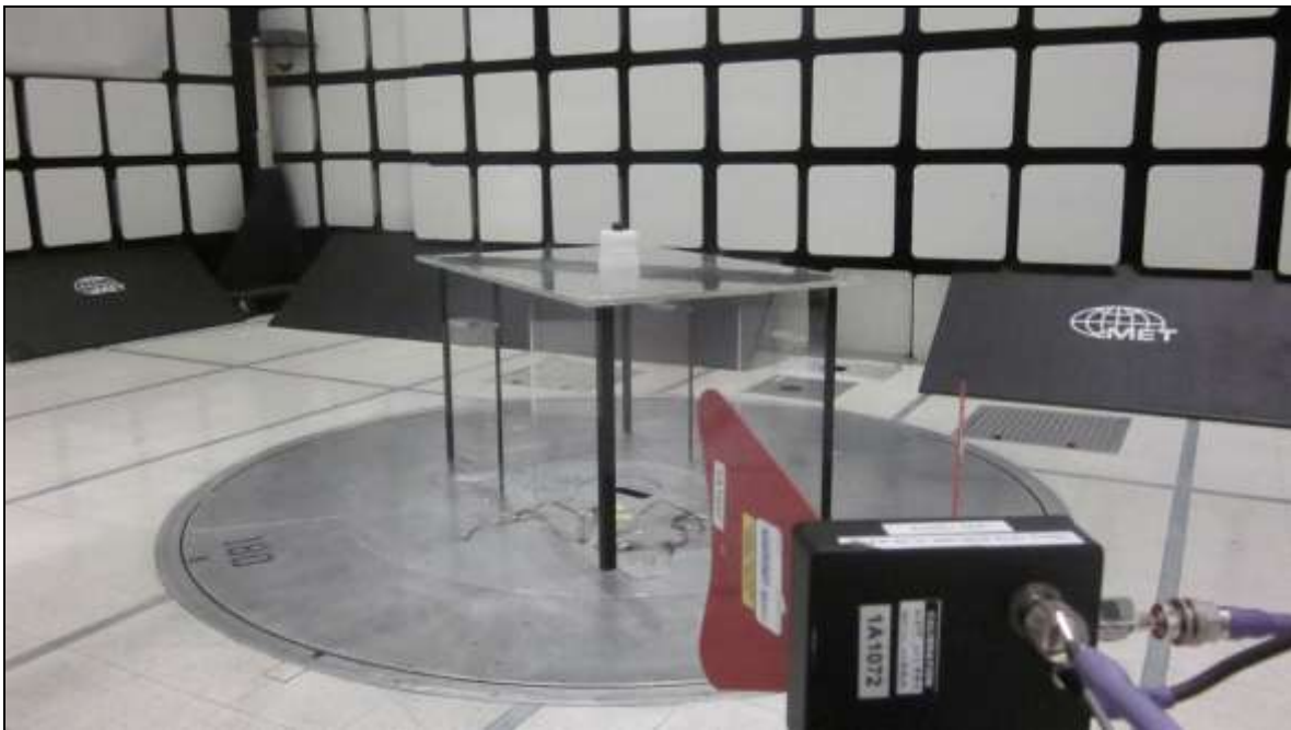
Photograph 4. Radiated Emissions, Test Setup, 1 GHz – 18 GHz
