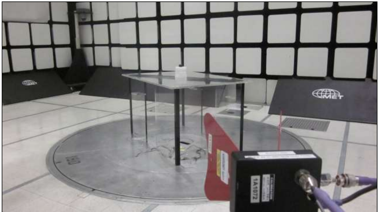
Photograph 2. Field Strength of Fundamental, Test Setup
