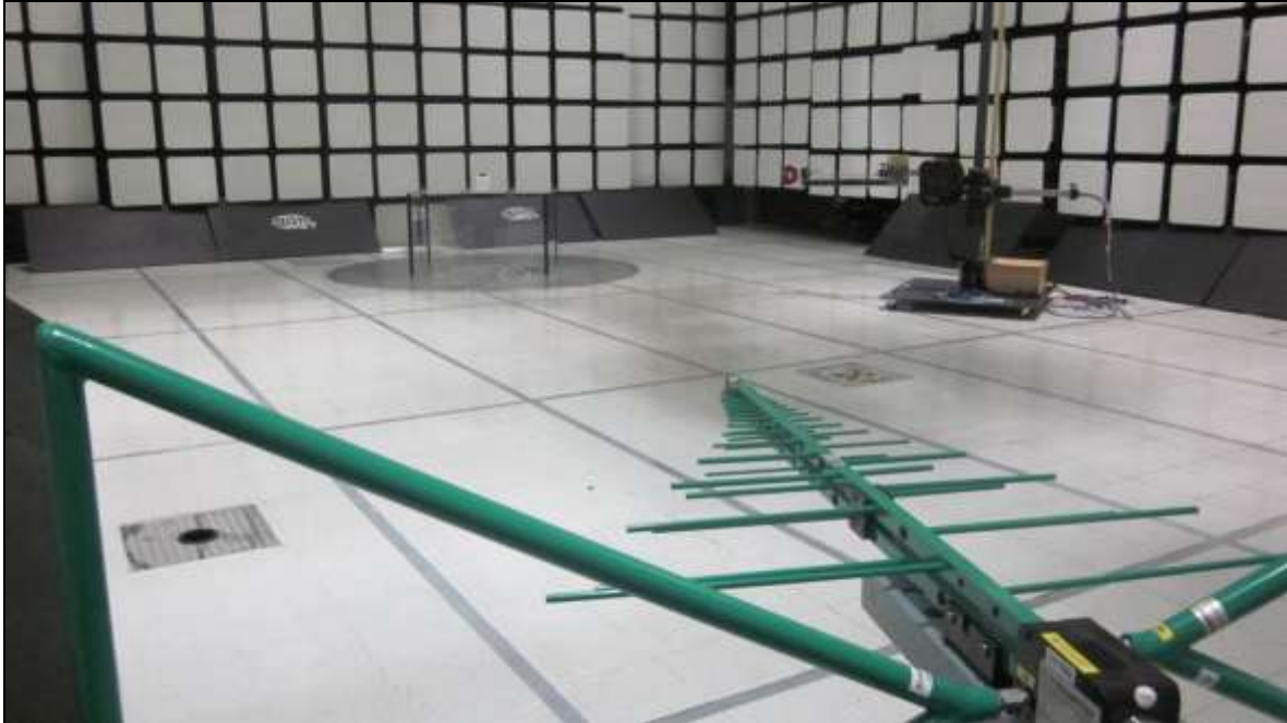
Photograph 3. Radiated Emissions, Test Setup, 30 MHz – 1 GHz
