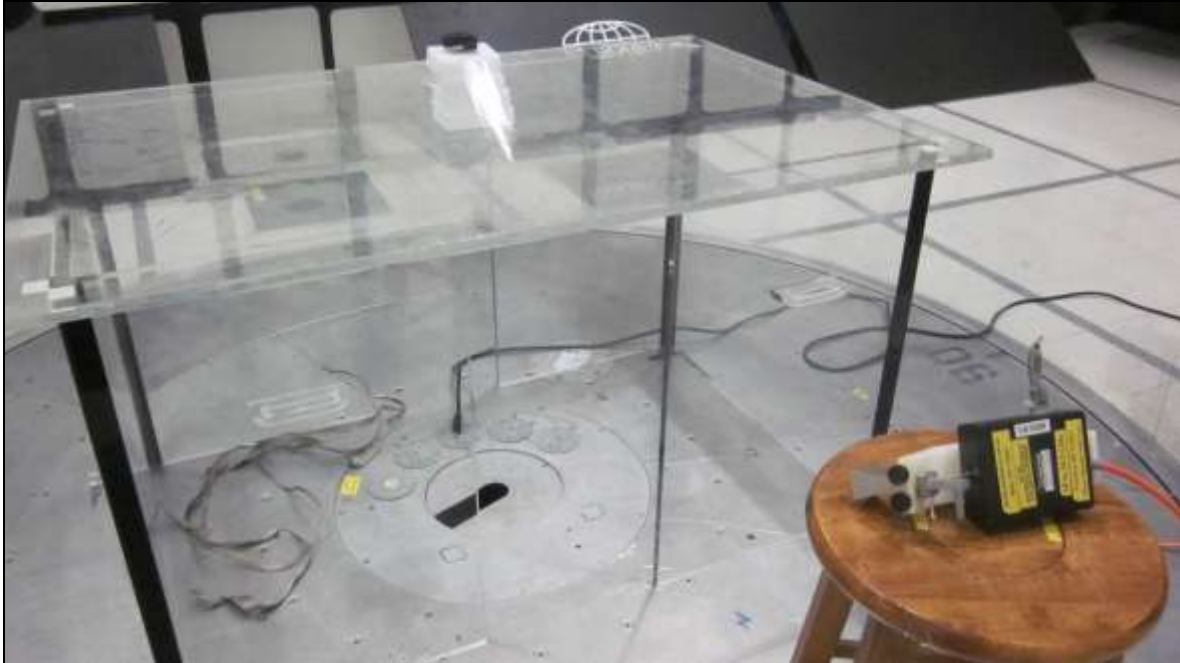
Photograph 5. Radiated Emissions, Test Setup, 18 GHz – 26 GHz
