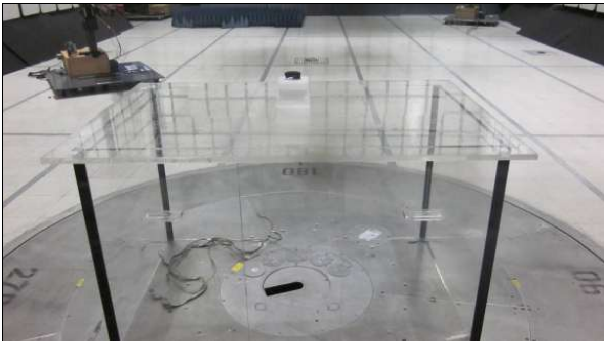
Photograph 6. Radiated Emissions, Test Setup, Rear View
