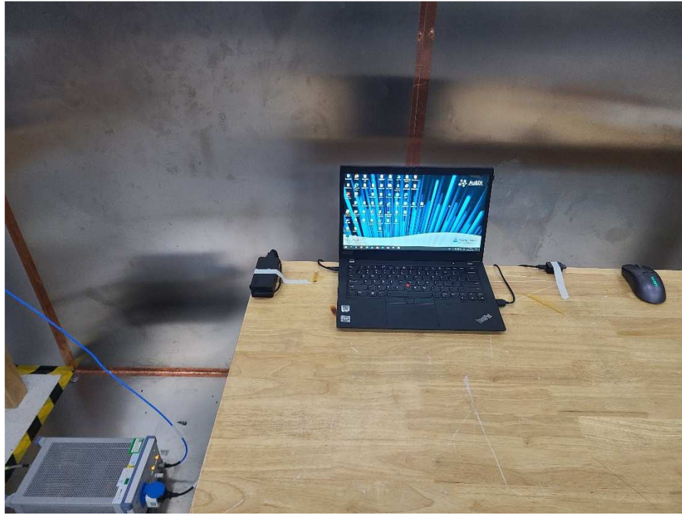
Photograph 3: Set-up for Conducted Emission on AC Mains
