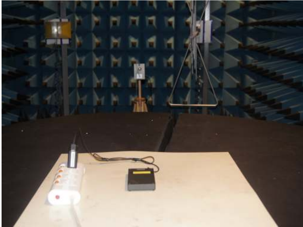
Photograph 6: Set-up for Conducted Emissions
