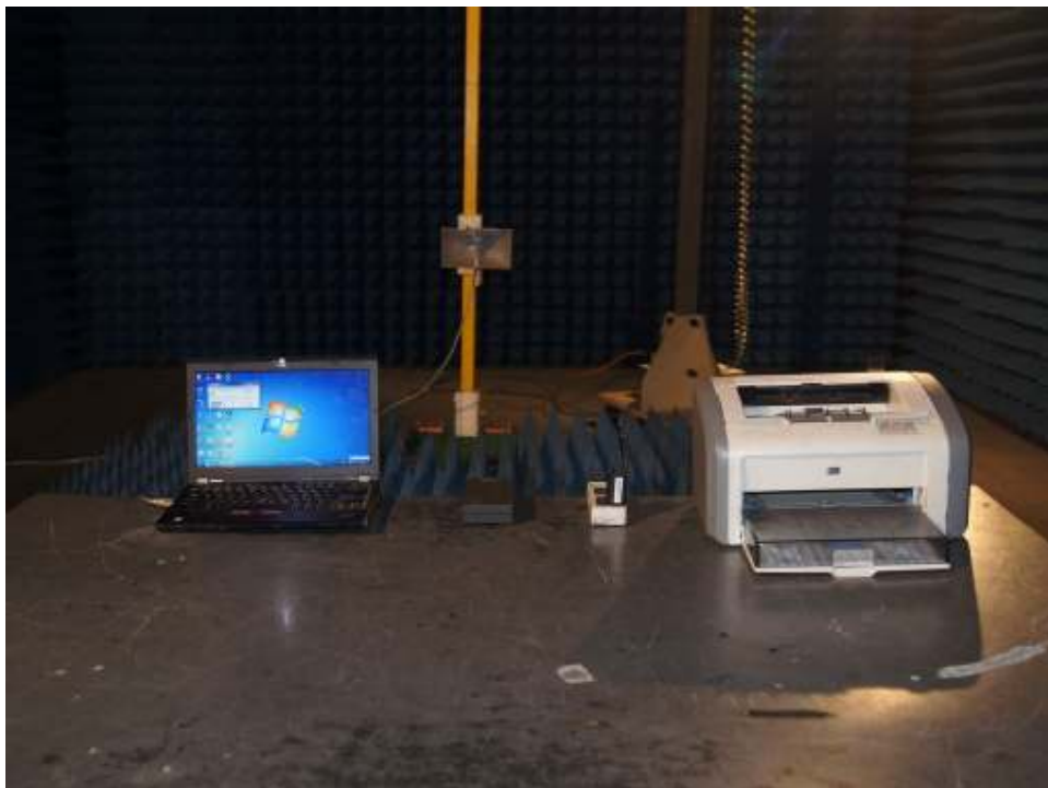
Photograph 8: Set-up for Radiated Emissions, above 1GHz
