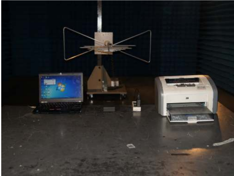
Photograph 8: Set-up for Radiated Emissions, above 1GHz
