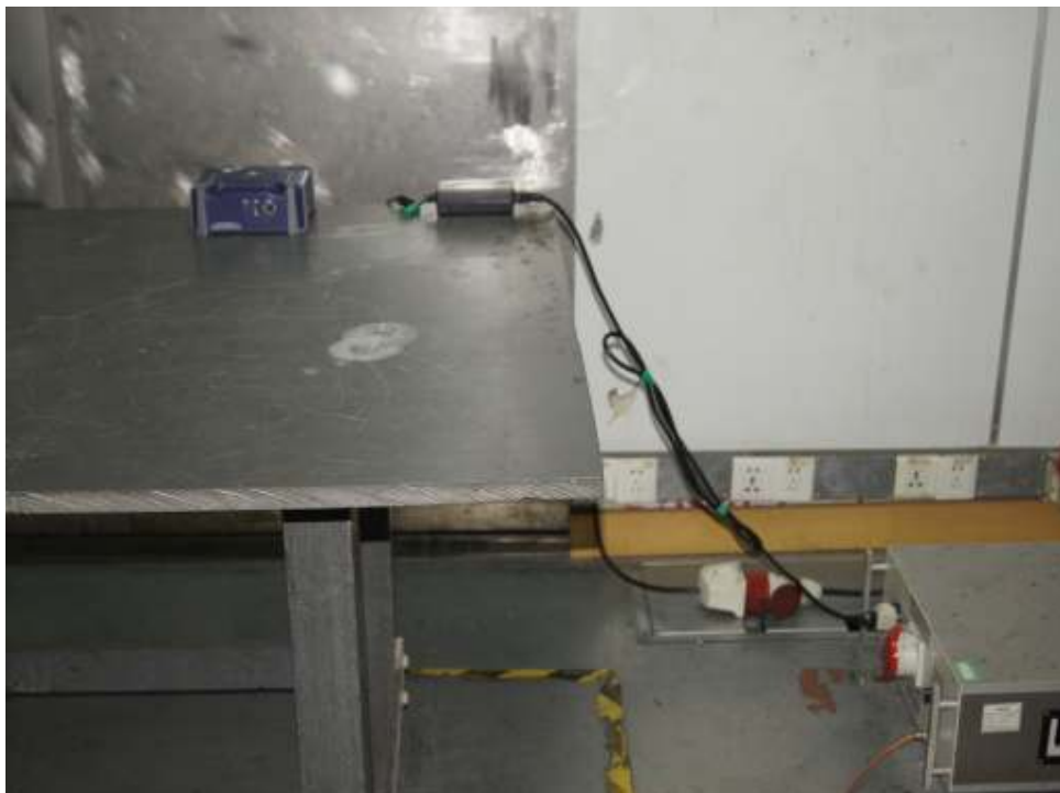
Photograph 6: Set-up for Conducted Emissions
