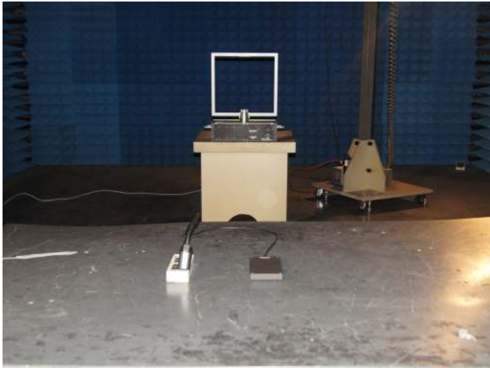
Photograph 2: Set-up for Spurious Emissions (30MHz-1GHz)
