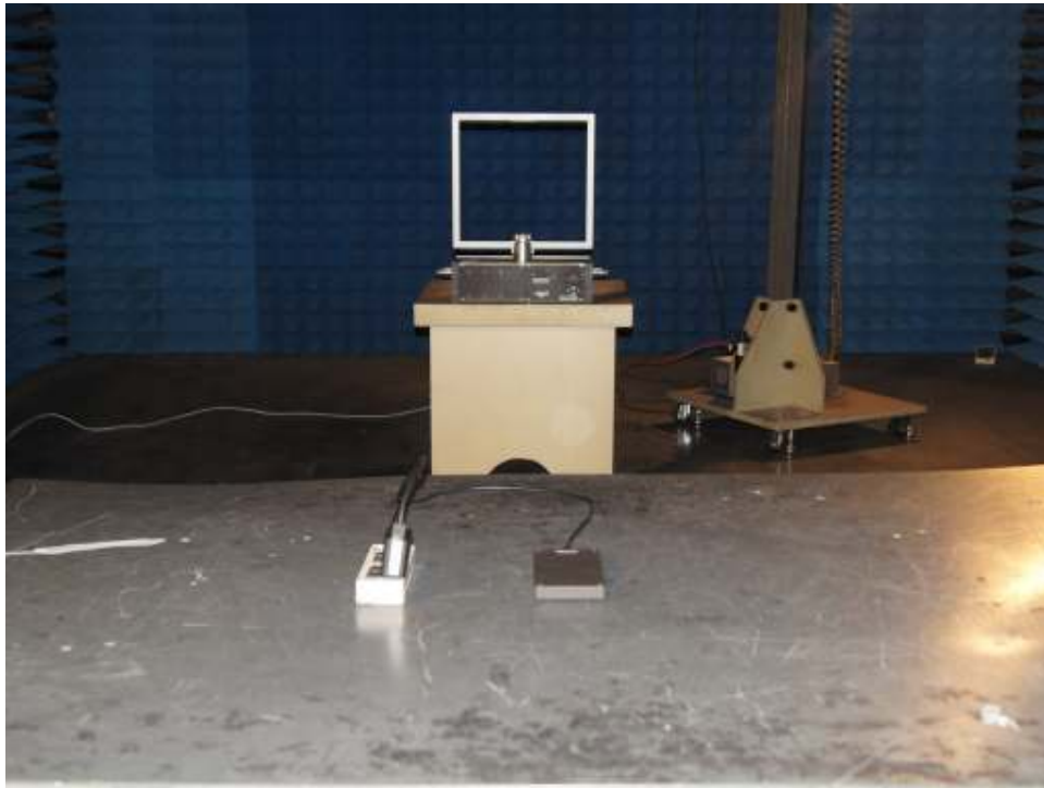
Photograph 2: Set-up for Spurious Emissions (30MHz-1GHz)
