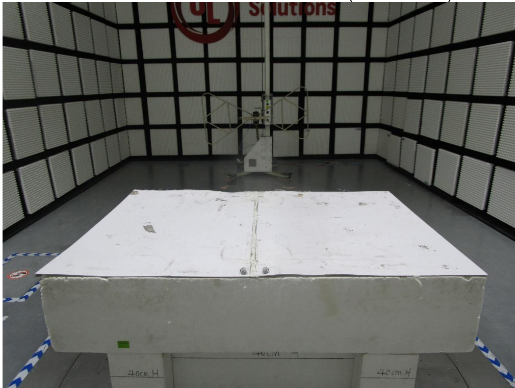
RADIATED RF MEASUREMENT SETUP (Below 30MHz)
