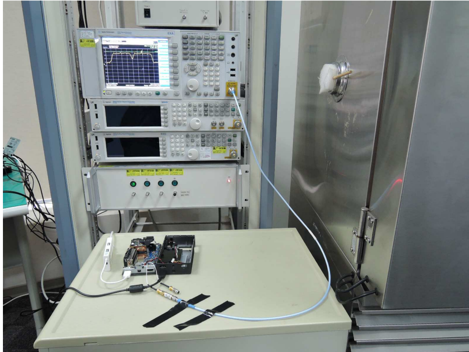
Photograph 4: Set-up for Conducted testing
