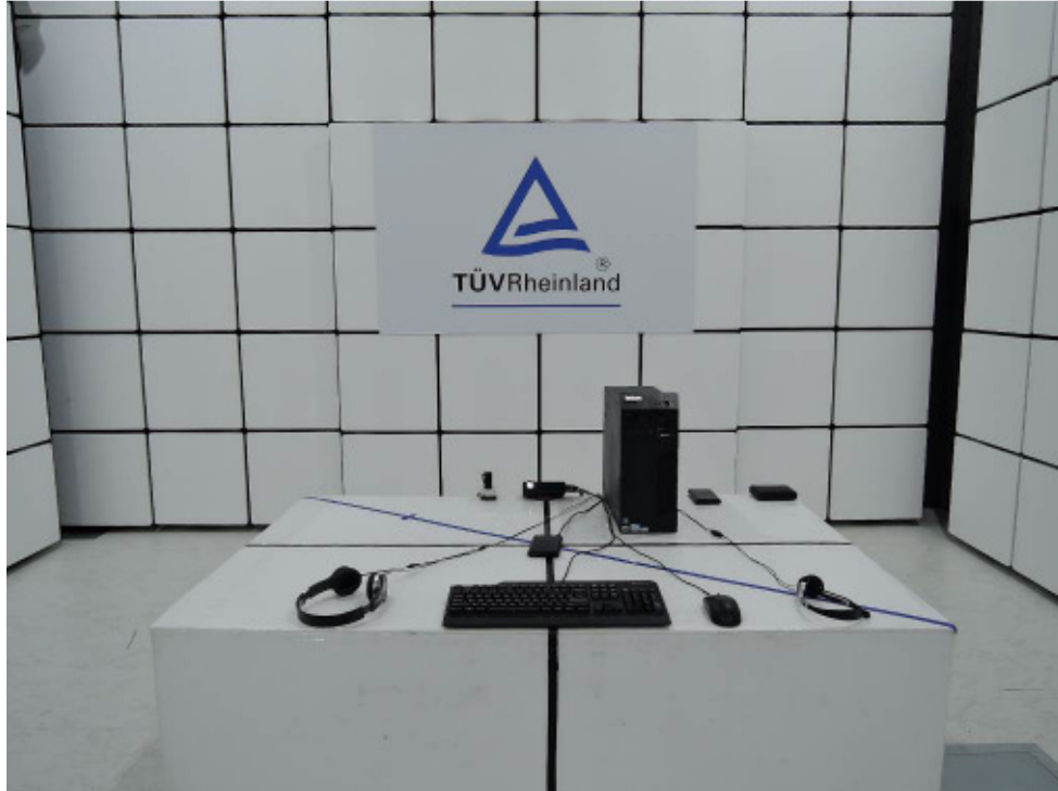
Picture 3: Radiated Emission, 30 - 1000 MHz (Mode B)
