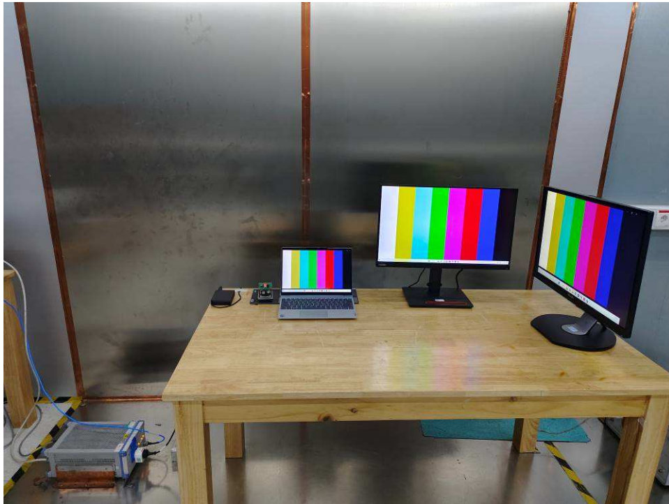
Photograph 1: Set-up for Conducted Emission on AC Mains
