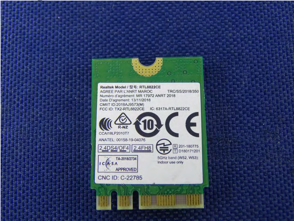
(18) EUT Photo WLAN Card : Realtek / RTL8822CE
