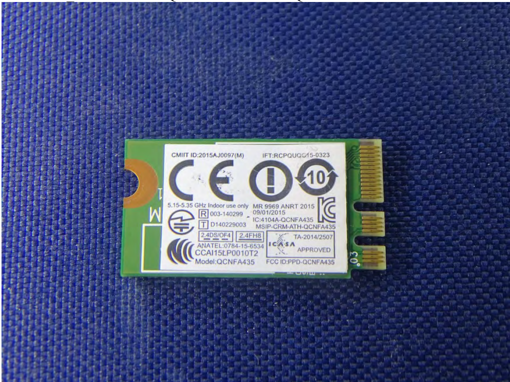
(20) EUT Photo WLAN Card : Qualcomm Atheros / QCNFA435
