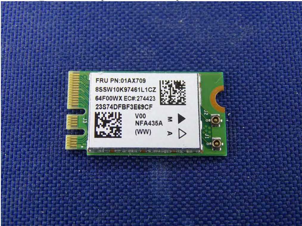
(19) EUT Photo WLAN Card : Qualcomm Atheros / QCNFA435
