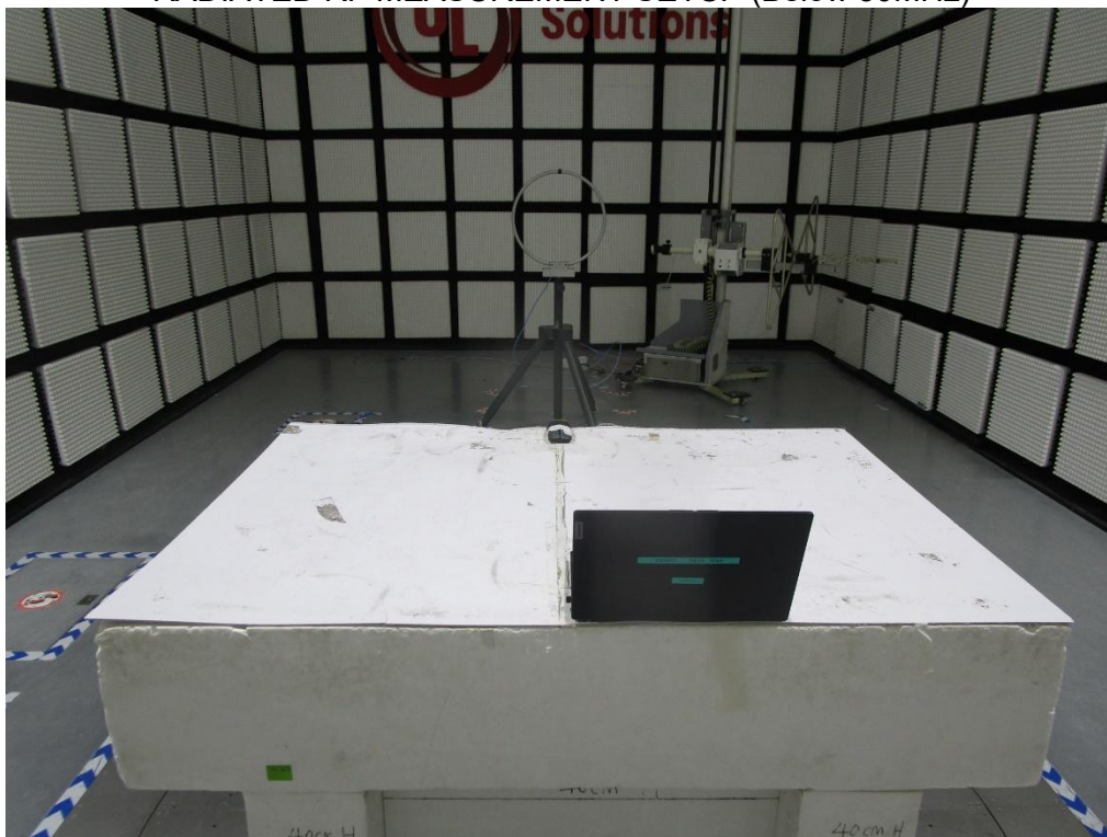
RADIATED RF MEASUREMENT SETUP (Below 30MHz)
