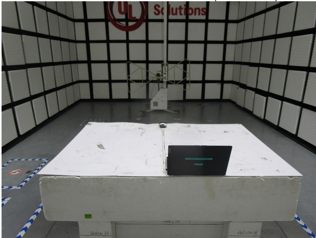
RADIATED RF MEASUREMENT SETUP (Below 30MHz)
