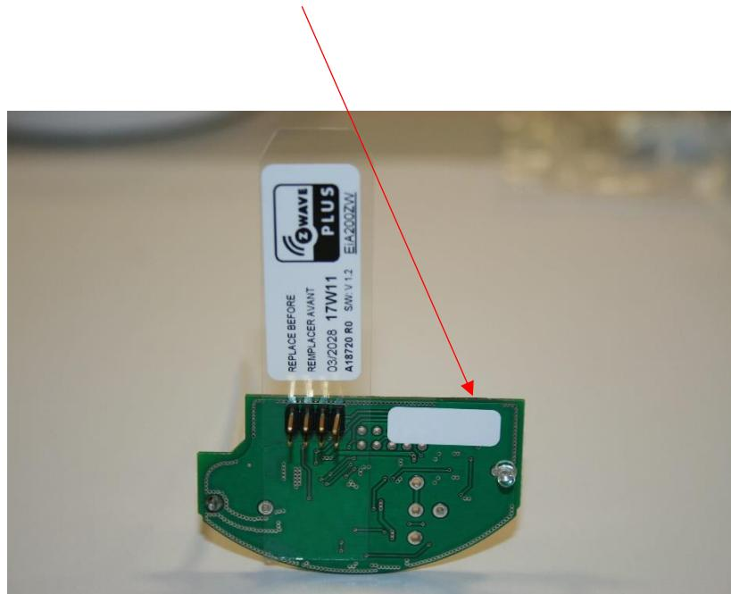
FCC/ISED label to be placed on outside rim of Host Alarm
