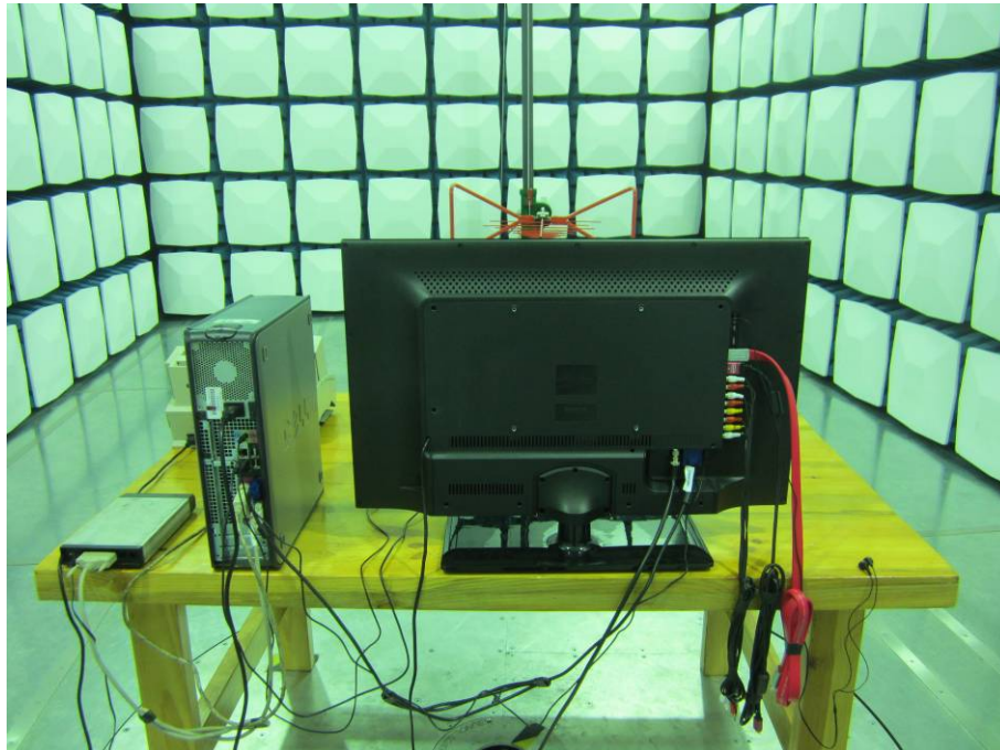
Below 1GHz: Radiated Emissions - Rear View
