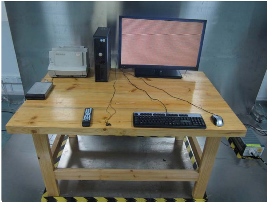
Conduction Emissions - Front View
