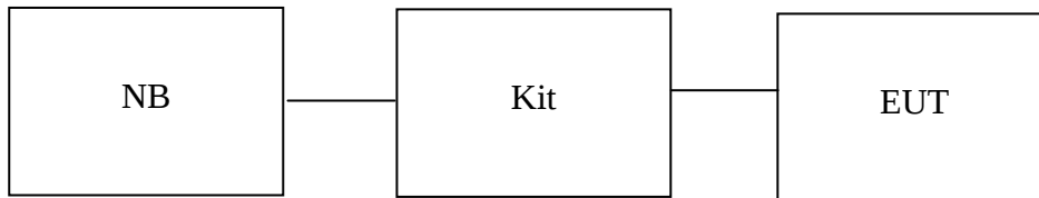
Fig. 1 Radiated/Conducted Emission Configuration
