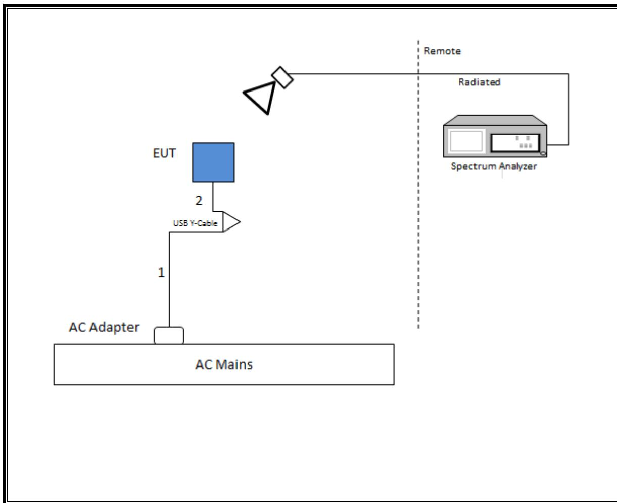
**SETUP DIAGRAM FOR LINE CONDUCTED TEST**
