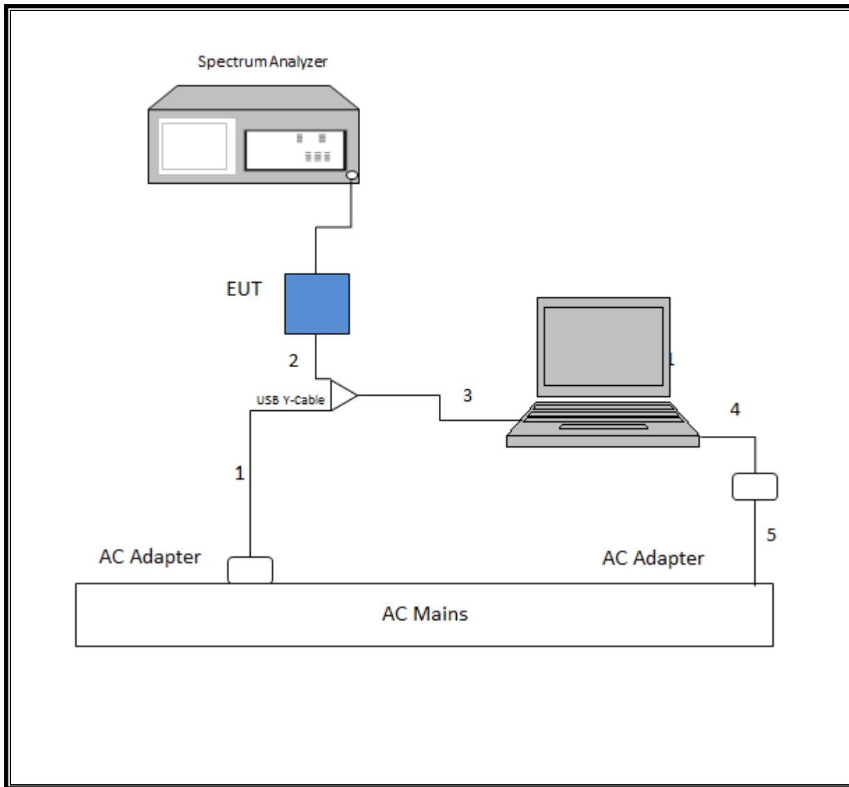
**SETUP DIAGRAM FOR RADIATED TESTS**
