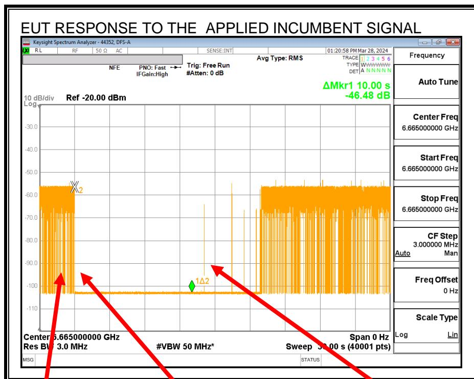
Transmissions cease while the Incumbent AWGN Signal is present and resume after it is removed.
