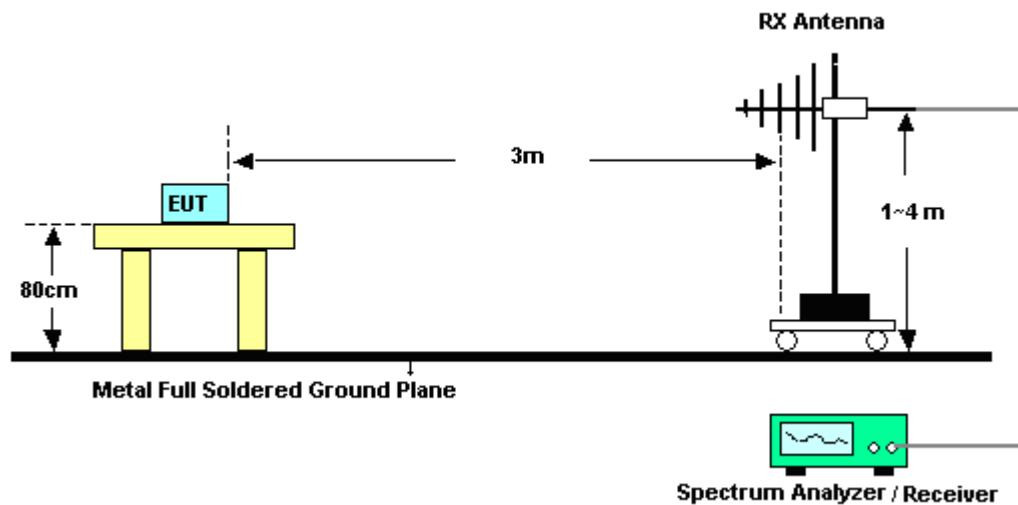
For radiated test from 1GHz to 18GHz
