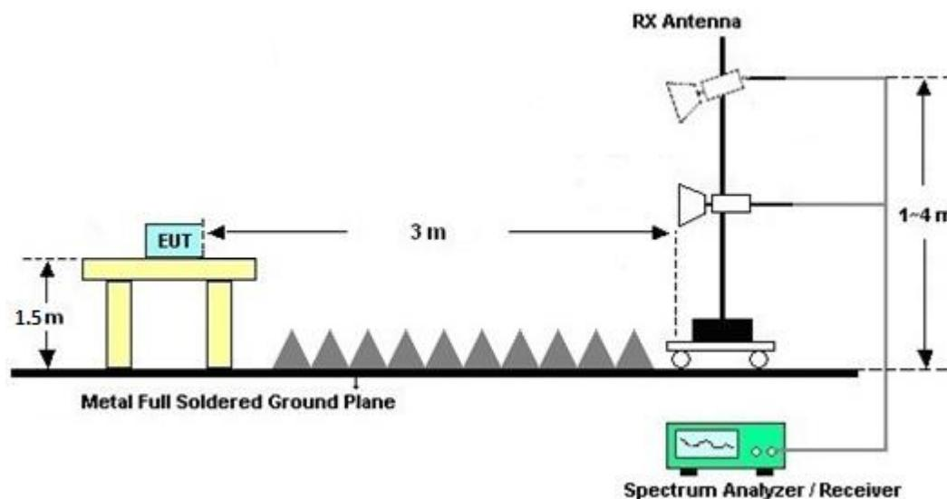
For radiated test above 18GHz
