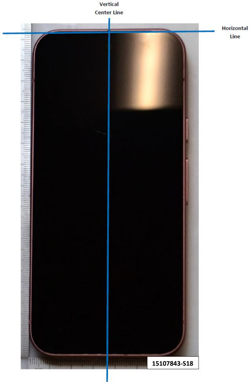
Photograph 4: Handset Vertical and Horizontal Reference Lines
