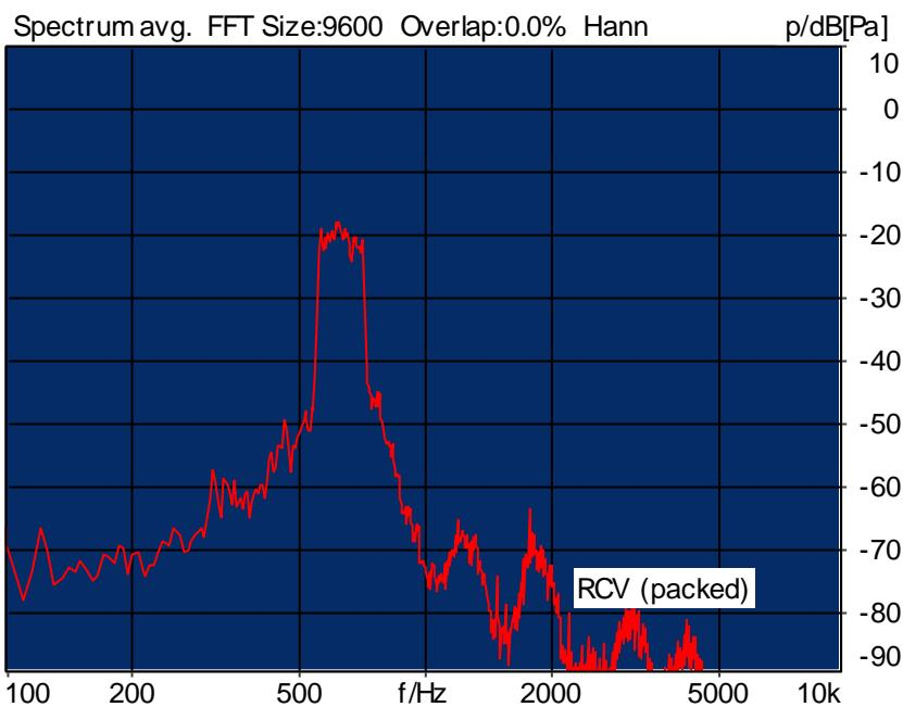
Distortion (Noise) RCV (packed): 30.42 dB (3.01%) Ok
