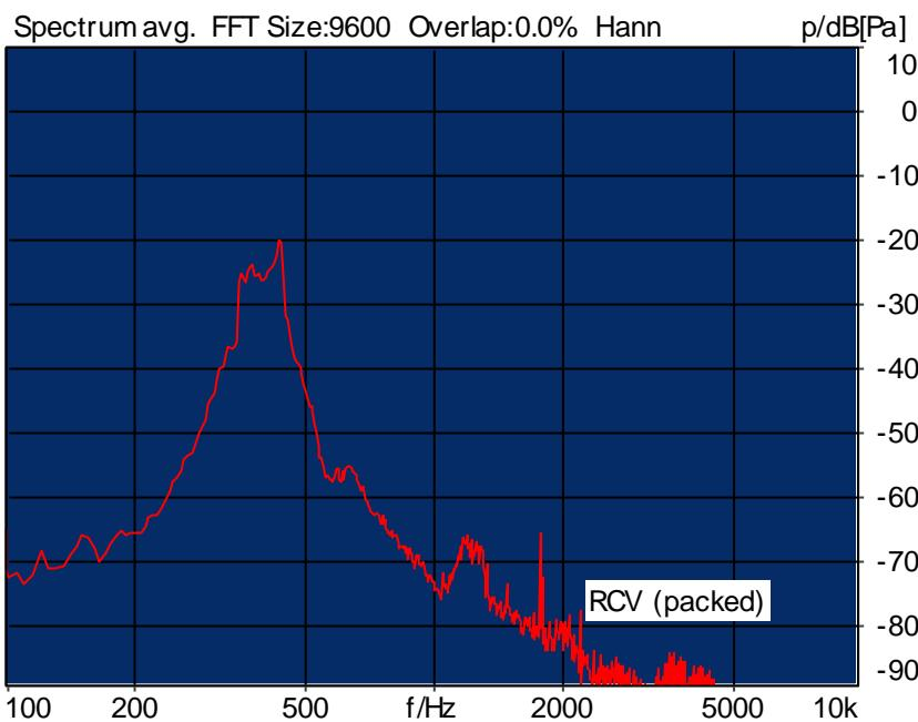
Distortion (Noise) RCV (packed): 24.19 dB (6.17%) Ok
