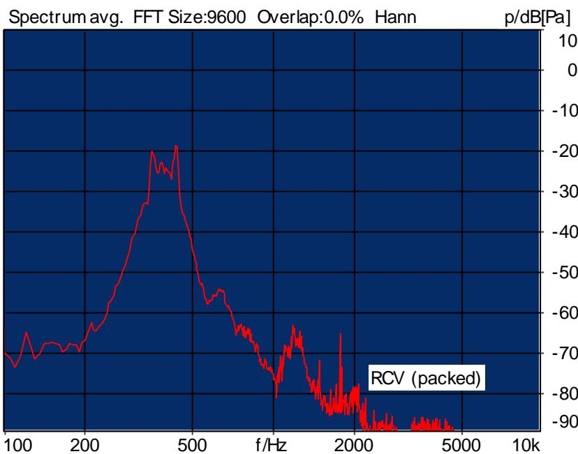
Distortion (Noise) RCV (packed): 25.21 dB (5.49%) Ok
