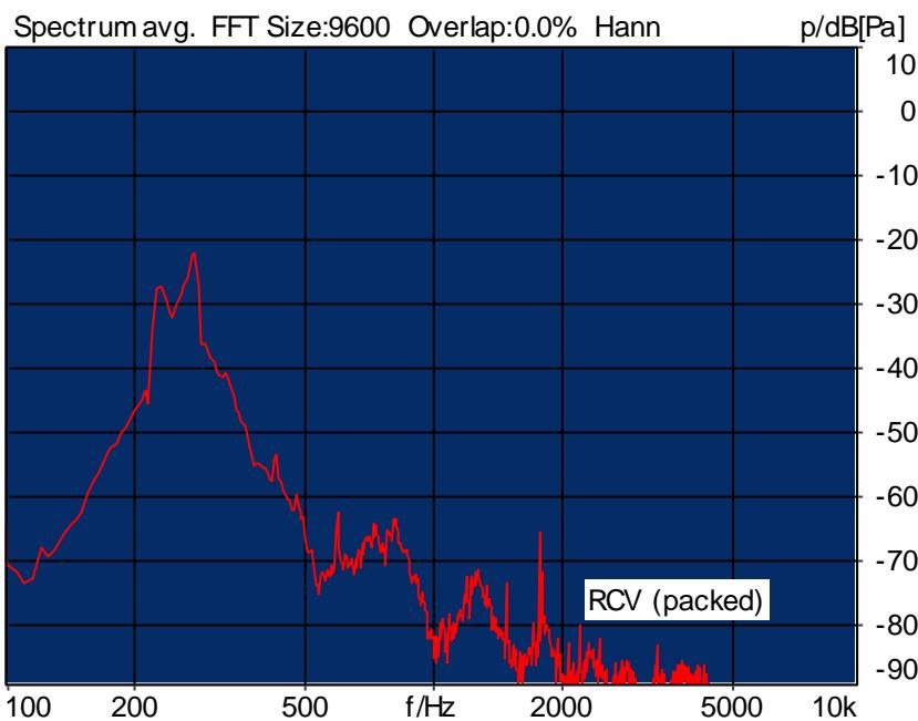
Distortion (Noise) RCV (packed): 23.51 dB (6.68%) Ok
