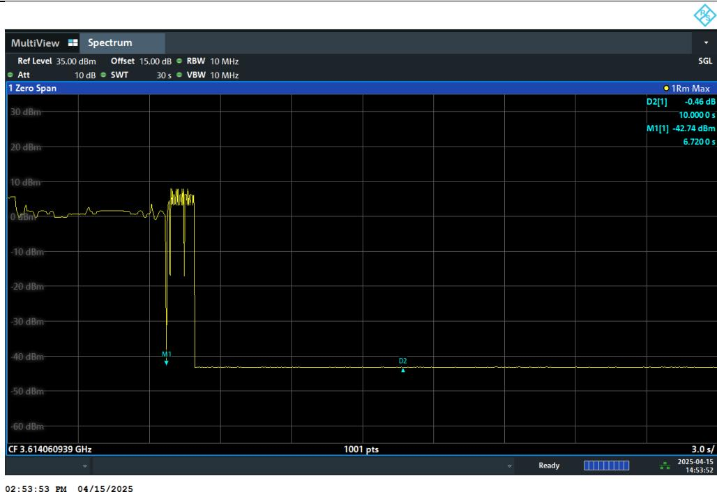
**[Step 5] Configure SAS granted CBSD to operate at frequency 3670-3690 MHz & power level 20 dBm/MHz**
