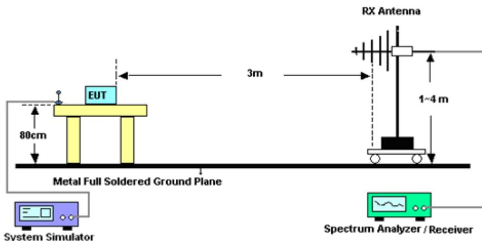
For radiated emissions from 1GHz to 18GHz
