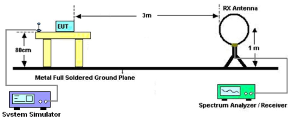
For radiated emissions from 30MHz to 1GHz
