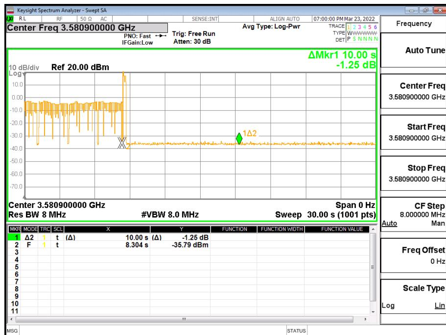
**[Step 5] Setup with 3670-3690MHz & power level 24dBm/MHz**
