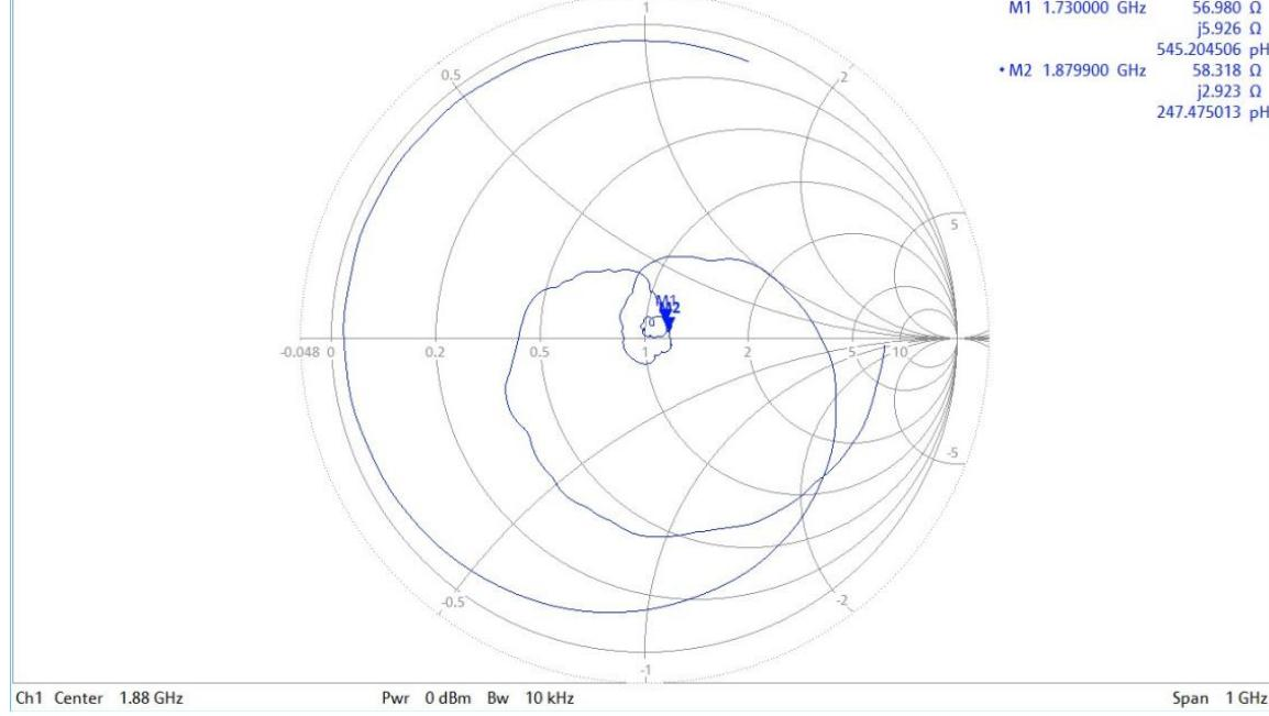
**<Dipole Verification Data> - CD1880 V3, serial no. 1038 (Data of Measurement : 9.17.2020)**
