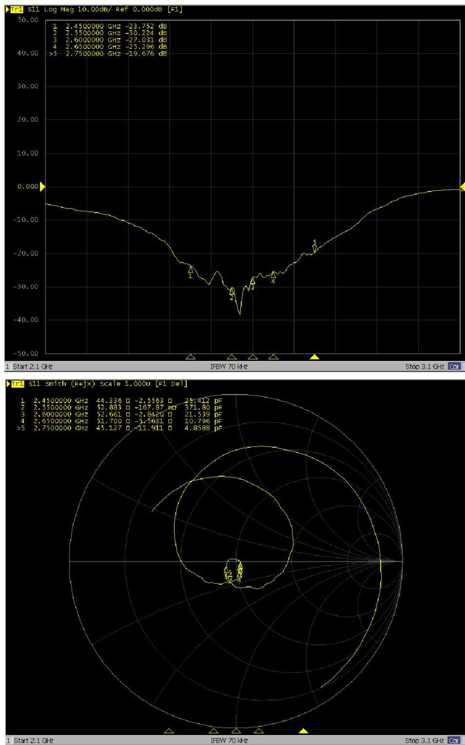
**<Dipole Verification Data> - CD2600 V3, serial no. 1010 (Data of Measurement : 3.12.2021)**
