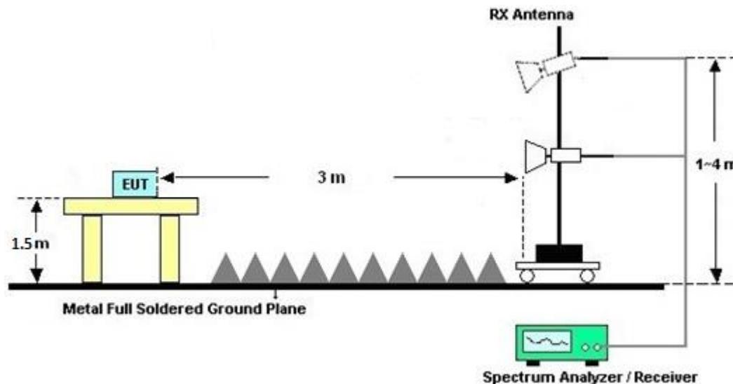
For radiated test above 18GHz
