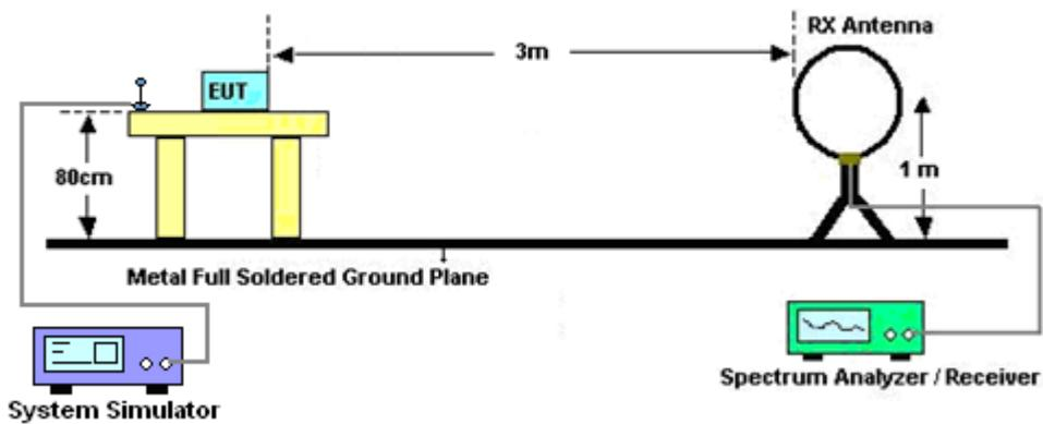
For radiated emissions from 30MHz to 1GHz
