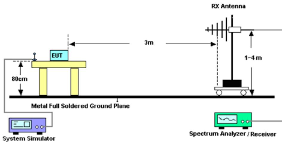
For radiated emissions from 1GHz to 18GHz
