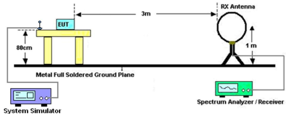
For radiated test from 30MHz to 1GHz
