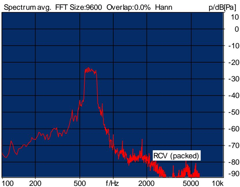
Distortion (Noise) RCV (packed): 25.30 dB (5.43%) Ok
