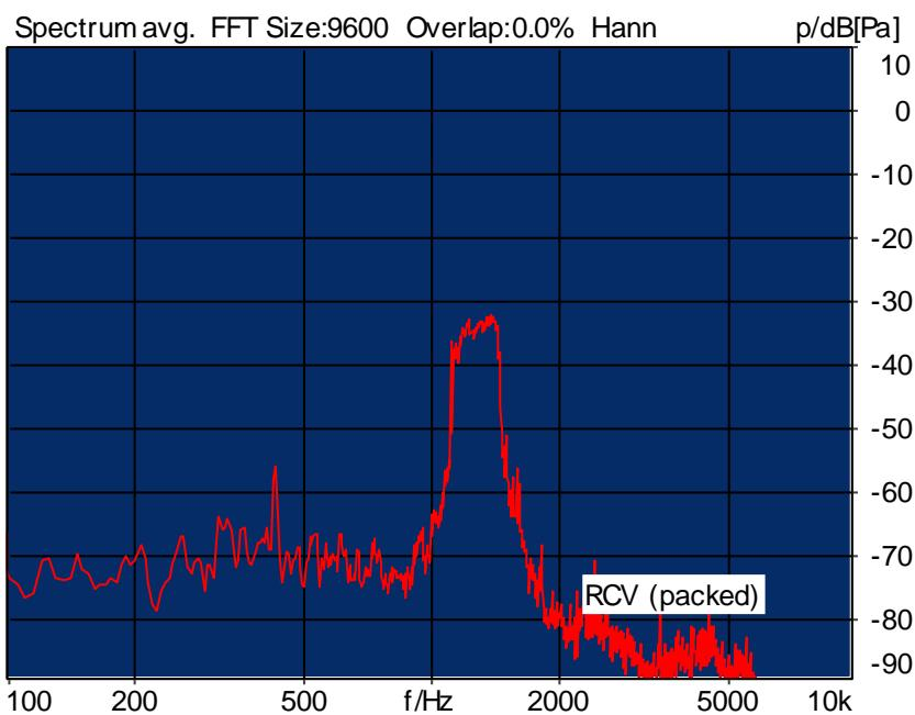
Distortion (Noise) RCV (packed): 22.46 dB (7.54%) Ok
