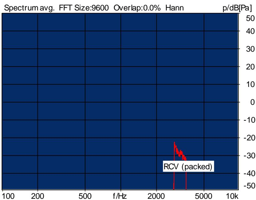
Distortion (Noise) RCV (packed): 38.66 dB (1.17%) Ok
