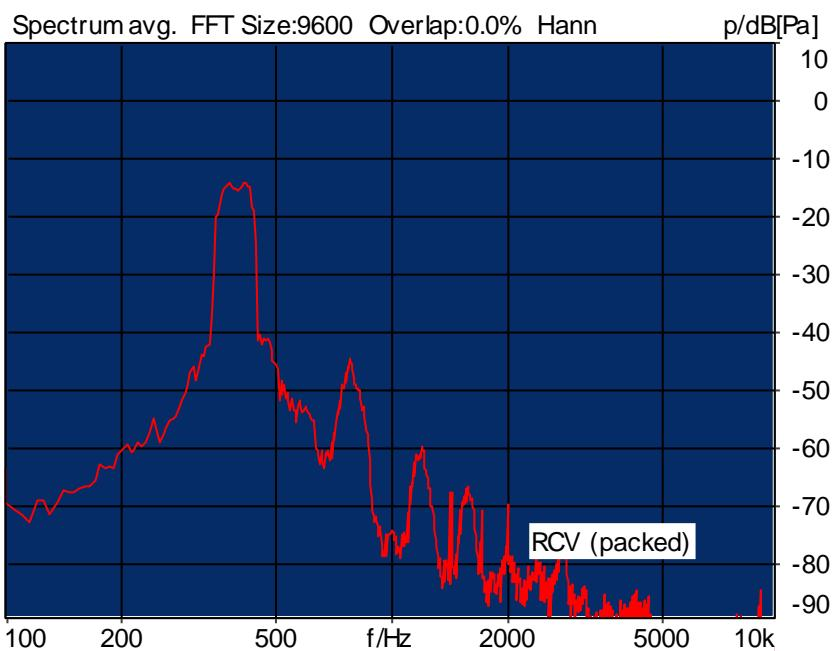
Distortion (Noise) RCV (packed): 30.22 dB (3.08%) Ok
