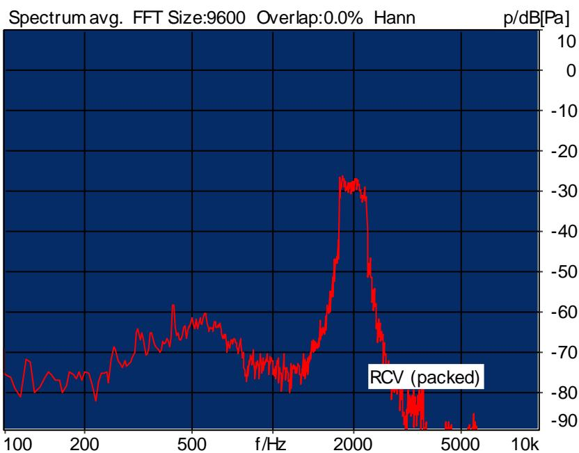
Distortion (Noise) RCV (packed): 23.61 dB (6.60%) Ok
