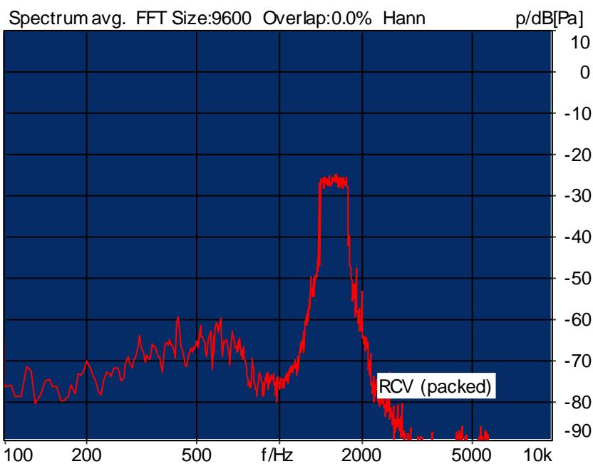
Distortion (Noise) RCV (packed): 26.59 dB (4.68%) Ok
