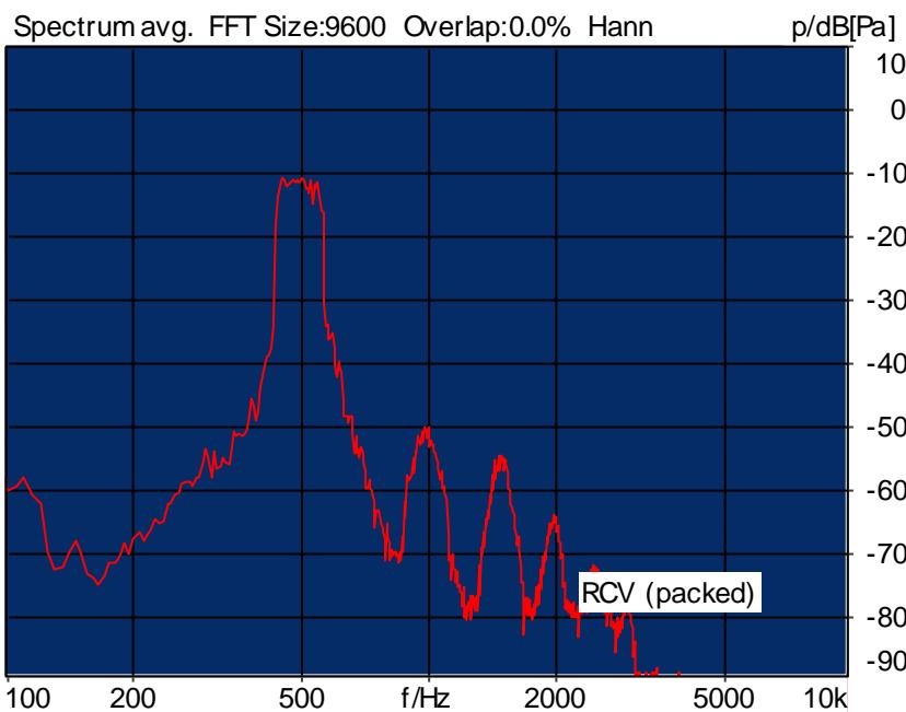
Distortion (Noise) RCV (packed): 33.40 dB (2.14%) Ok
