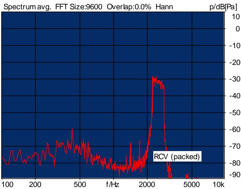
Distortion (Noise) RCV (packed): 30.34 dB (3.04%) Ok
