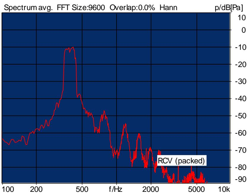
Distortion (Noise) RCV (packed): 32.57 dB (2.35%) Ok
