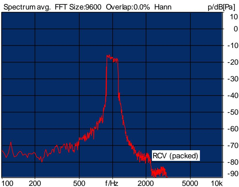
Distortion (Noise) RCV (packed): 31.80 dB (2.57%) Ok
