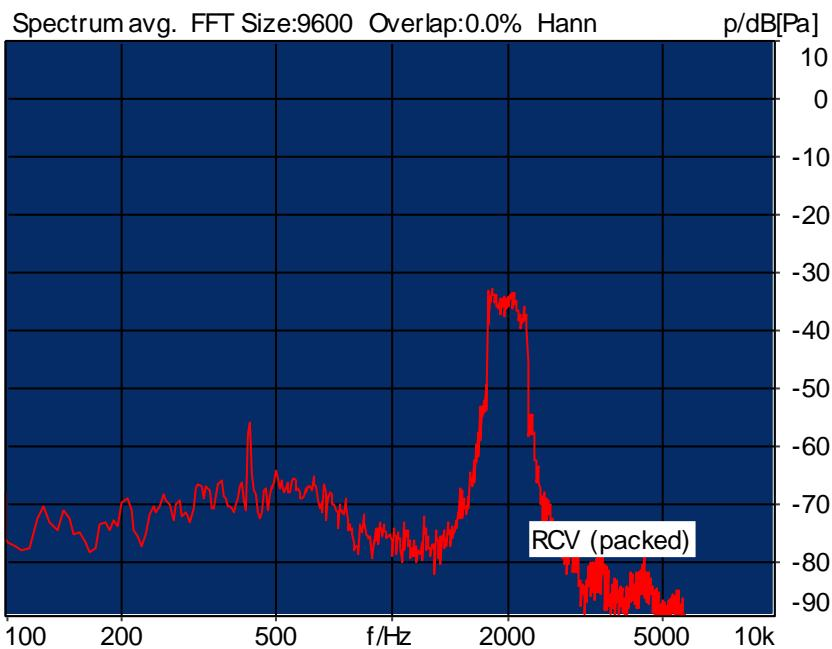
Distortion (Noise) RCV (packed): 23.35 dB (6.80%) Ok
