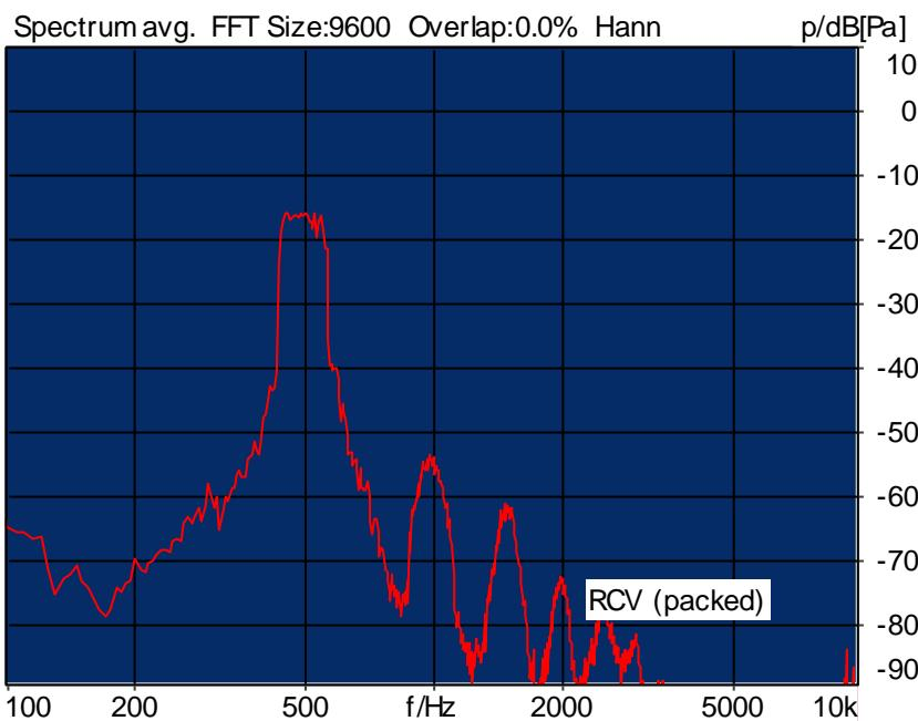
Distortion (Noise) RCV (packed): 33.46 dB (2.12%) Ok
