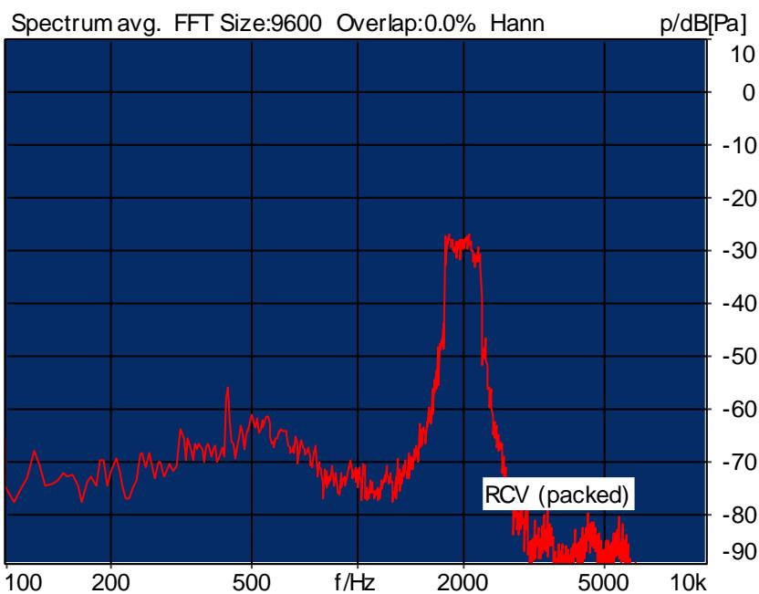
Distortion (Noise) RCV (packed): 23.77 dB (6.48%) Ok
