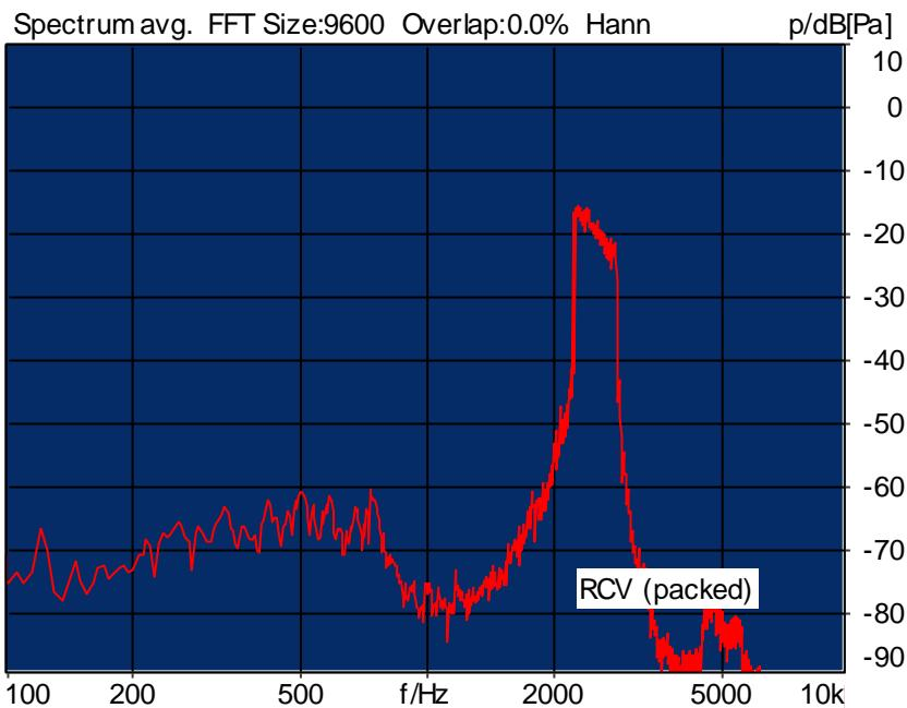
Distortion (Noise) RCV (packed): 31.87 dB (2.55%) Ok
