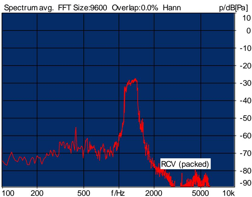
Distortion (Noise) RCV (packed): 21.83 dB (8.10%) Ok
