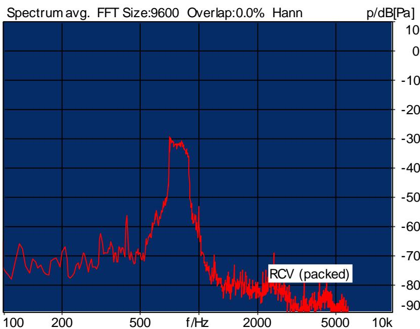
Distortion (Noise) RCV (packed): 24.88 dB (5.70%) Ok
