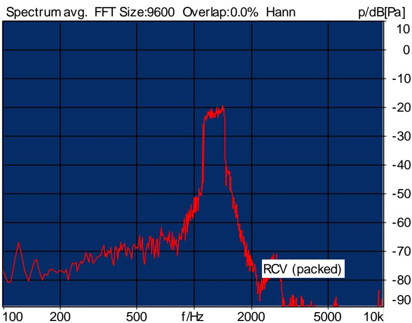
Distortion (Noise) RCV (packed): 23.54 dB (6.65%) Ok
