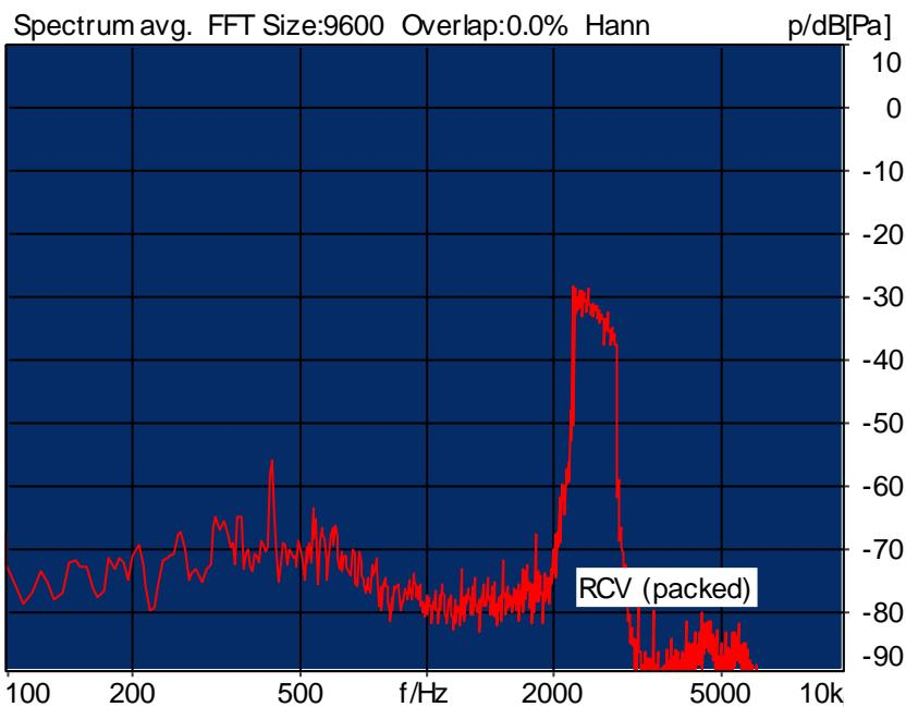
Distortion (Noise) RCV (packed): 29.53 dB (3.34%) Ok
