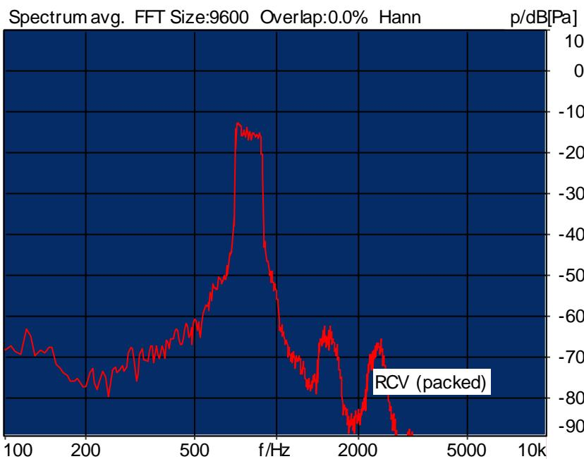
Distortion (Noise) RCV (packed): 35.96 dB (1.59%) Ok
