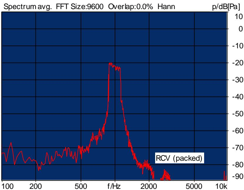
Distortion (Noise) RCV (packed): 30.19 dB (3.09%) Ok
