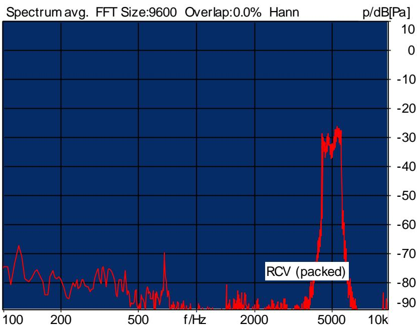
Distortion (Noise) RCV (packed): 34.35 dB (1.92%) Ok
