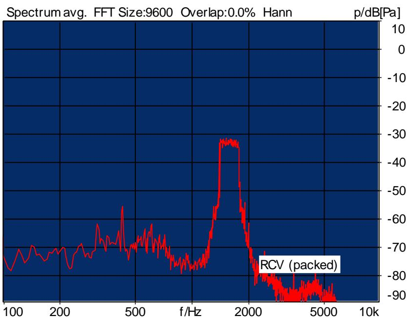
Distortion (Noise) RCV (packed): 25.56 dB (5.27%) Ok
