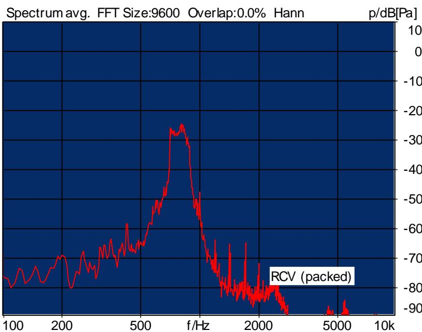
Distortion (Noise) RCV (packed): 24.61 dB (5.88%) Ok
