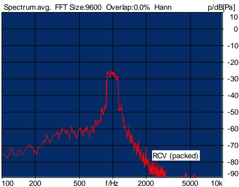
Distortion (Noise) RCV (packed): 22.66 dB (7.36%) Ok
