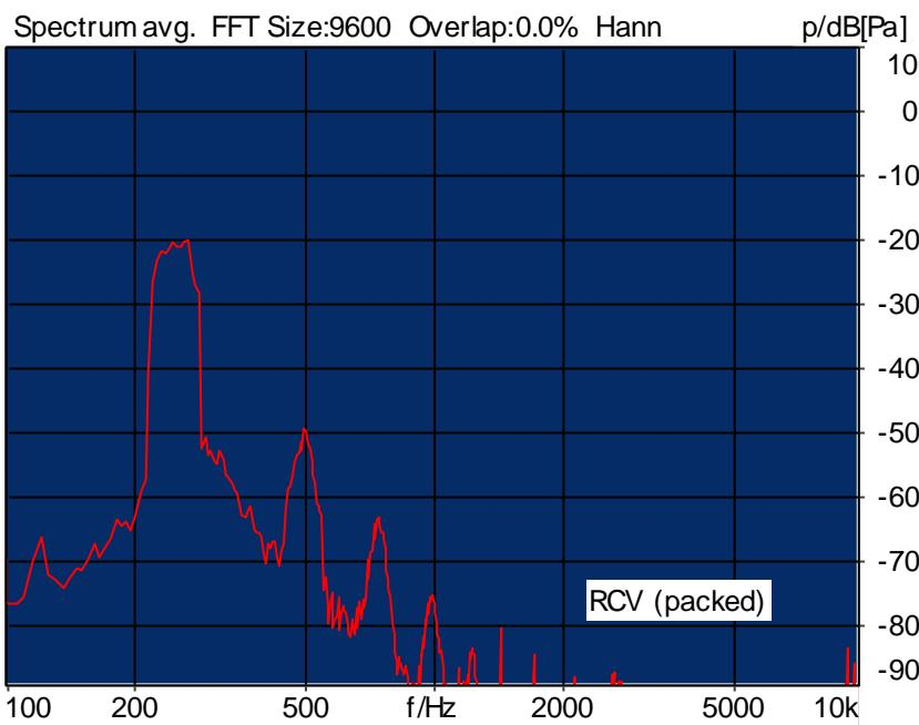
Distortion (Noise) RCV (packed): 32.53 dB (2.36%) Ok
