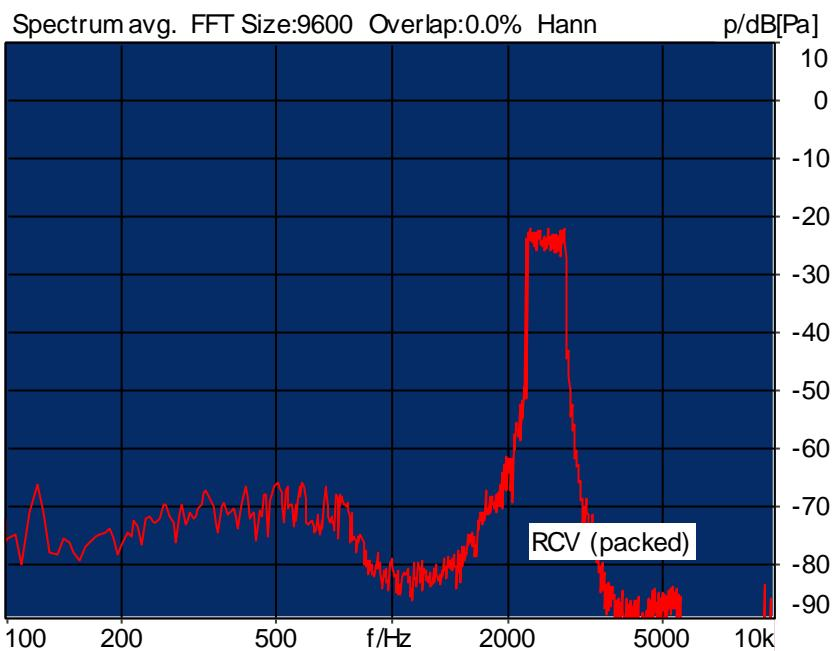
Distortion (Noise) RCV (packed): 30.55 dB (2.97%) Ok
