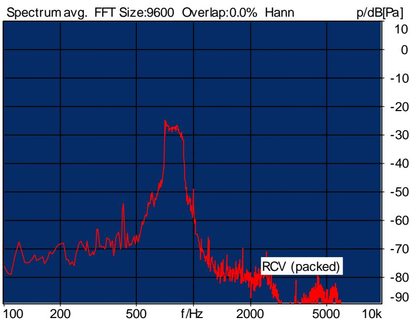
Distortion (Noise) RCV (packed): 25.17 dB (5.51%) Ok
