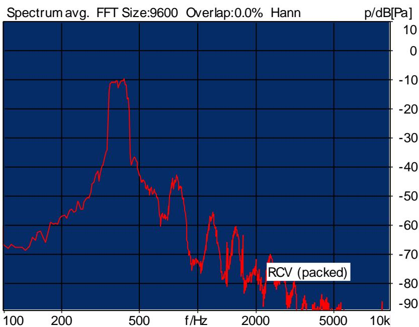
Distortion (Noise) RCV (packed): 30.89 dB (2.86%) Ok
