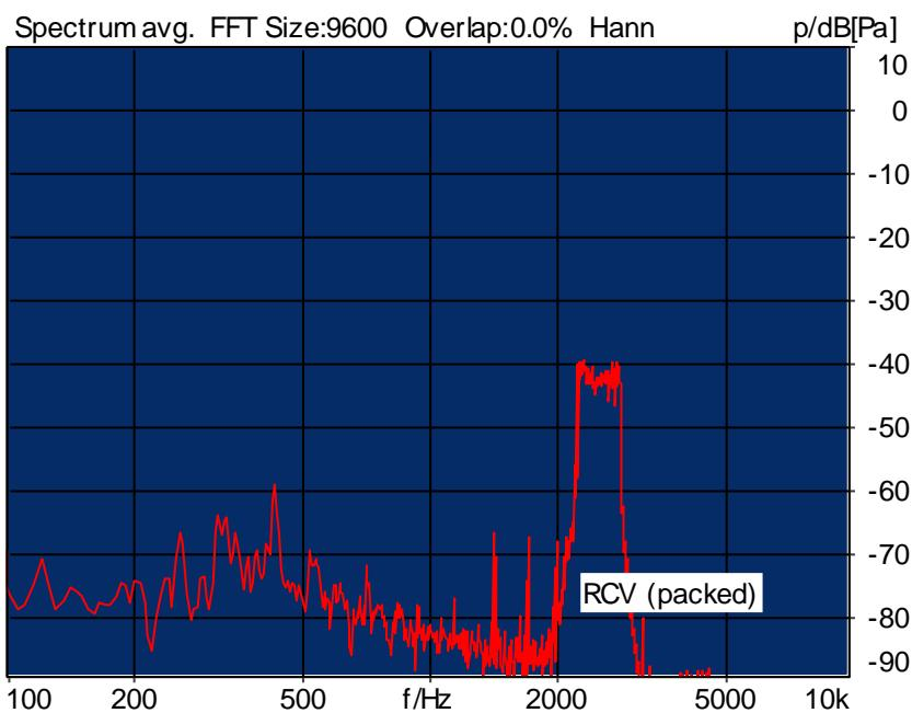
Distortion (Noise) RCV (packed): 26.72 dB (4.61%) Ok
