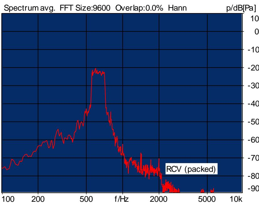
Distortion (Noise) RCV (packed): 26.40 dB (4.78%) Ok
