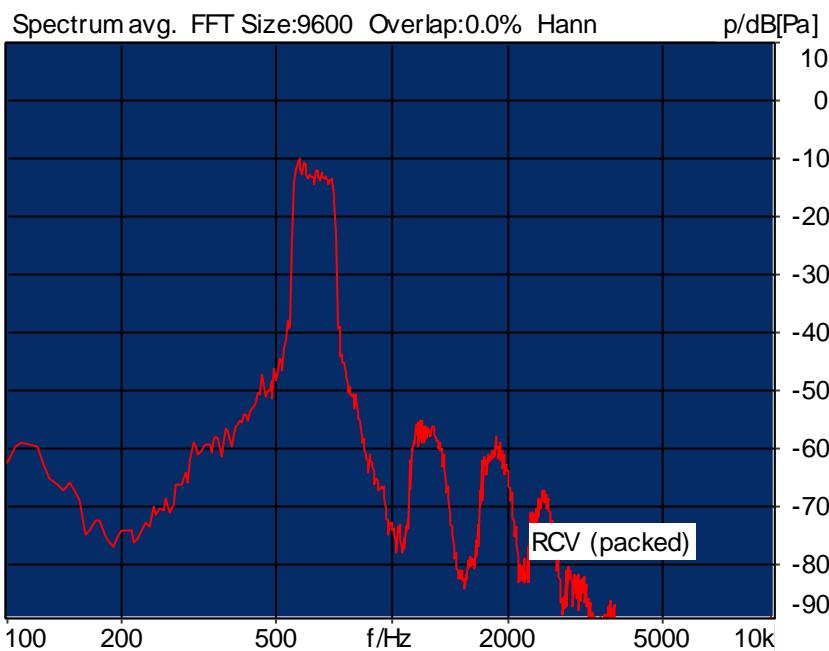
Distortion (Noise) RCV (packed): 35.99 dB (1.59%) Ok
