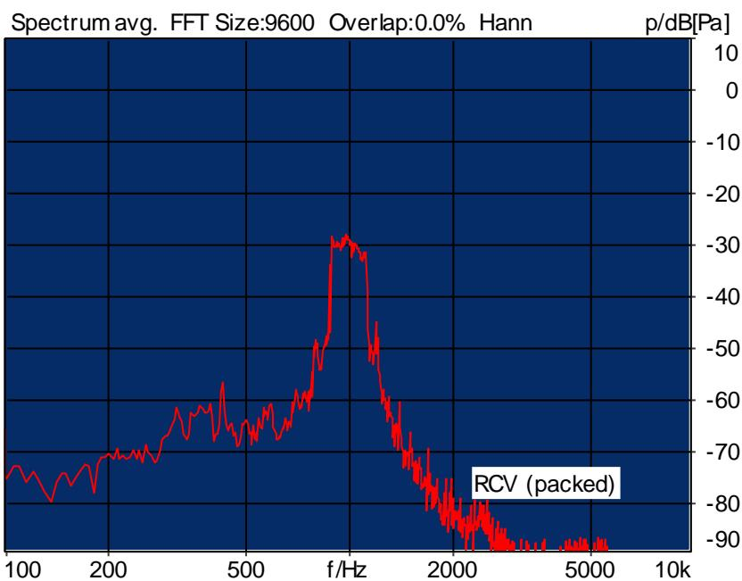
Distortion (Noise) RCV (packed): 21.88 dB (8.05%) Ok
