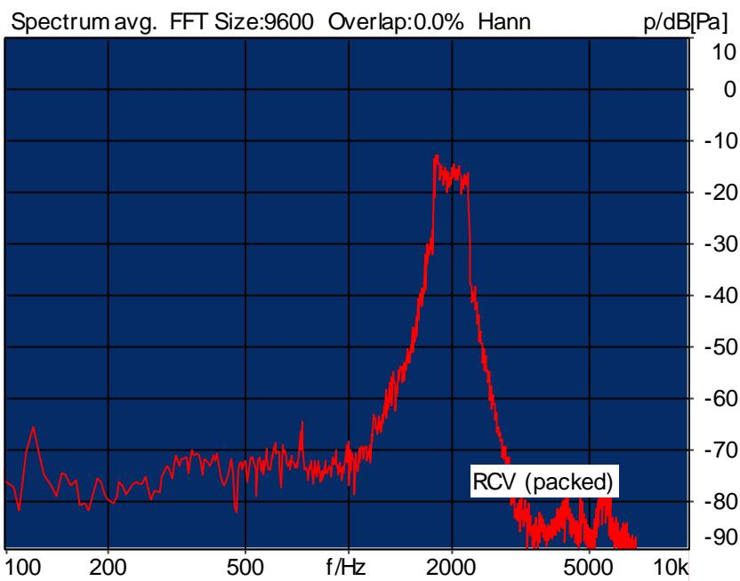
Distortion (Noise) RCV (packed): 20.82 dB (9.10%) Ok
