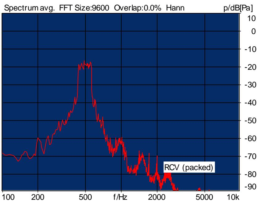
Distortion (Noise) RCV (packed): 27.73 dB (4.11%) Ok
