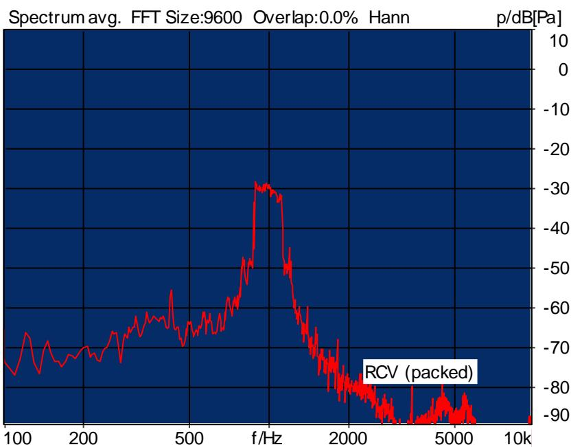
Distortion (Noise) RCV (packed): 21.19 dB (8.72%) Ok
