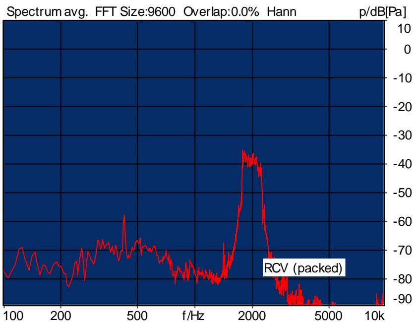
Distortion (Noise) RCV (packed): 21.79 dB (8.13%) Ok
