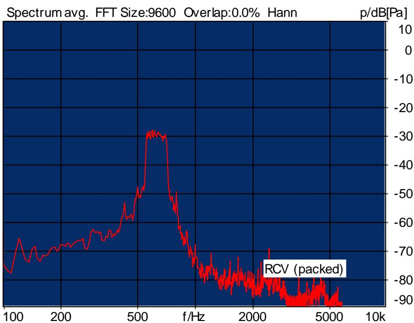
Distortion (Noise) RCV (packed): 24.95 dB (5.66%) Ok
