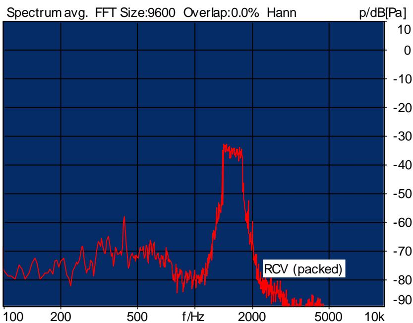
Distortion (Noise) RCV (packed): 23.14 dB (6.96%) Ok
