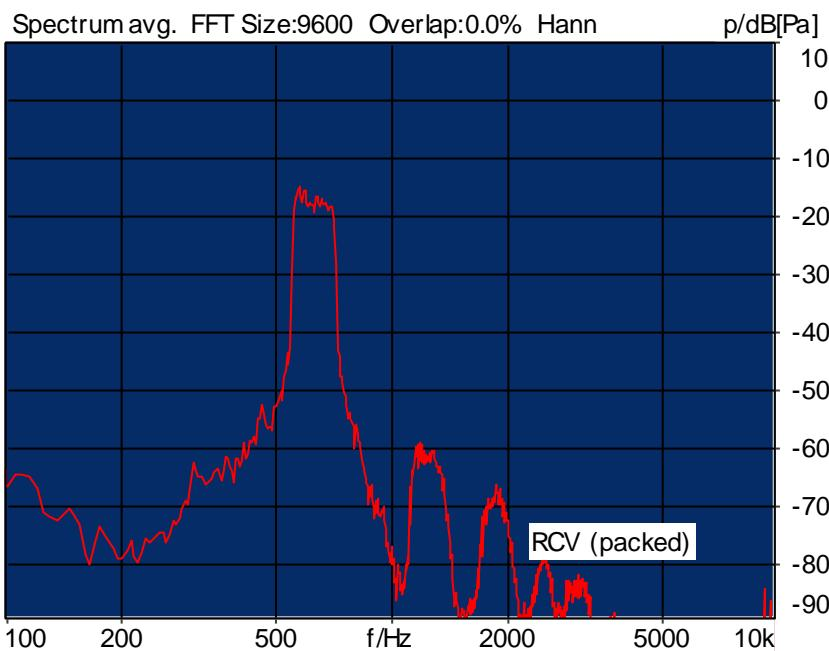
Distortion (Noise) RCV (packed): 36.55 dB (1.49%) Ok
