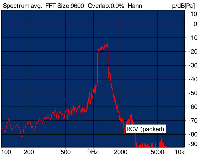
Distortion (Noise) RCV (packed): 22.28 dB (7.69%) Ok
