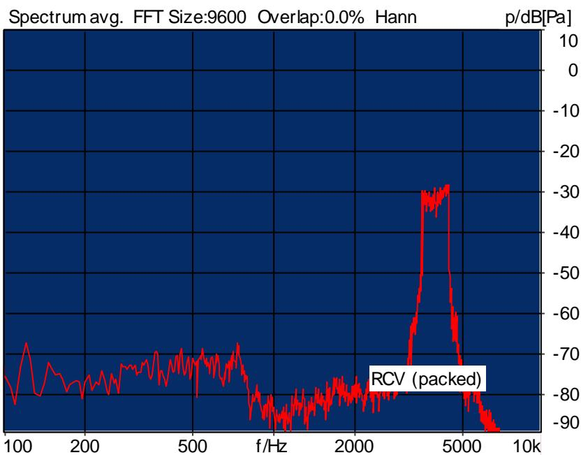
Distortion (Noise) RCV (packed): 27.81 dB (4.07%) Ok
