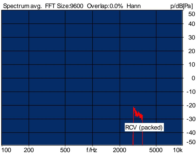
Distortion (Noise) RCV (packed): 40.97 dB (0.89%) Ok
