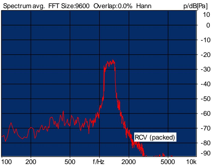
Distortion (Noise) RCV (packed): 22.88 dB (7.18%) Ok
