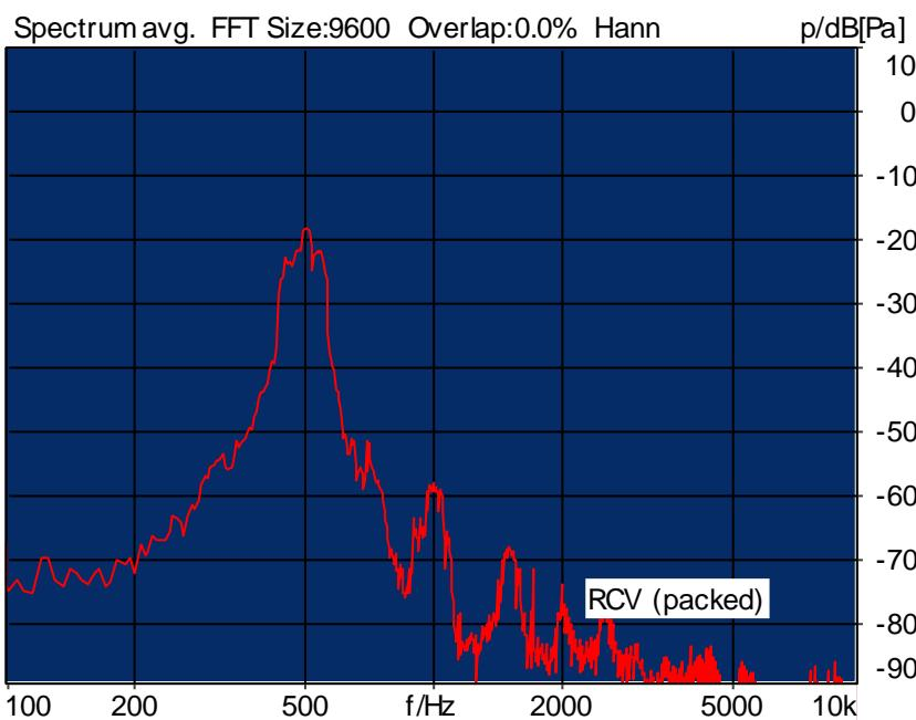
Distortion (Noise) RCV (packed): 28.75 dB (3.65%) Ok
