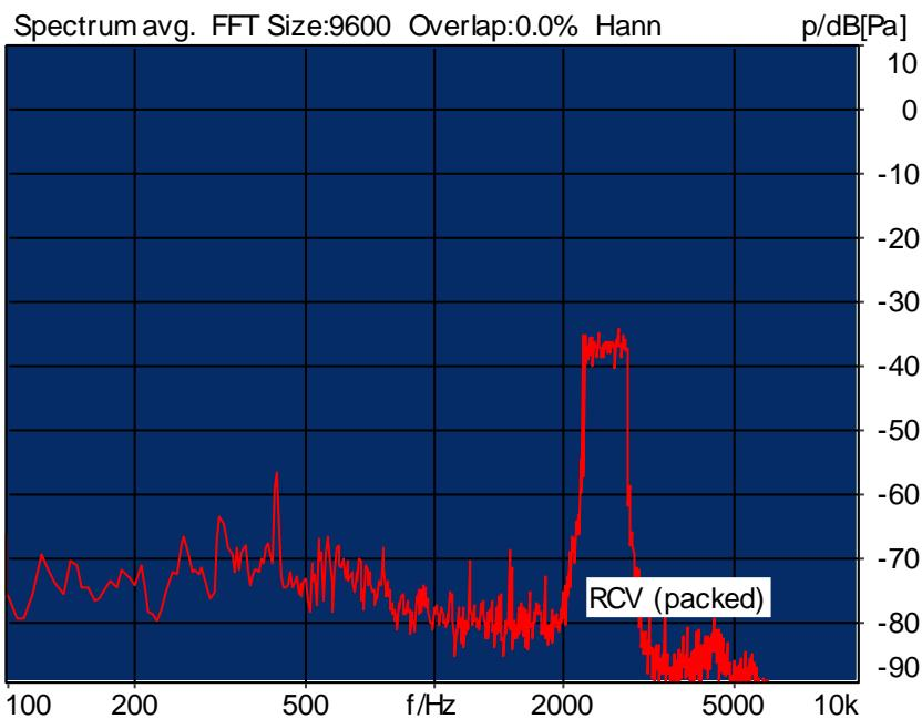
Distortion (Noise) RCV (packed): 29.18 dB (3.48%) Ok
