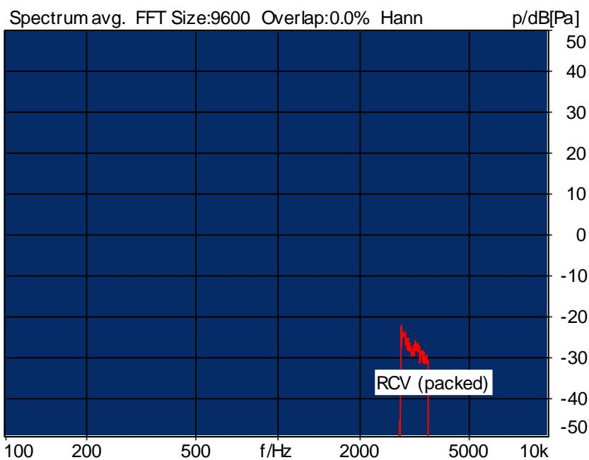
Distortion (Noise) RCV (packed): 40.76 dB (0.92%) Ok
