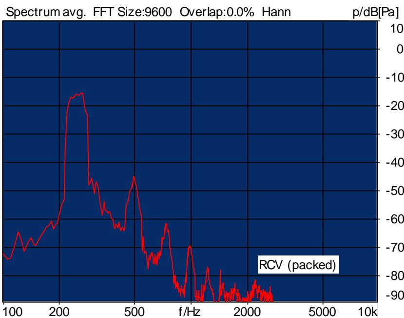
Distortion (Noise) RCV (packed): 33.15 dB (2.20%) Ok
