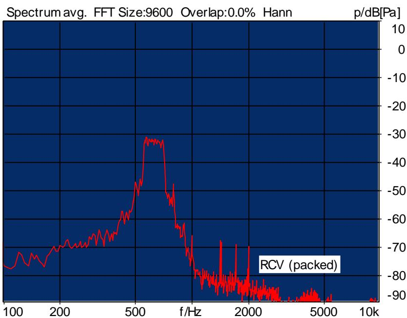
Distortion (Noise) RCV (packed): 21.69 dB (8.23%) Ok
