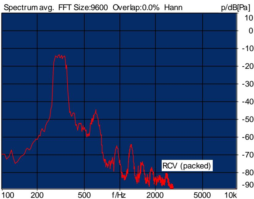
Distortion (Noise) RCV (packed): 32.50 dB (2.37%) Ok
