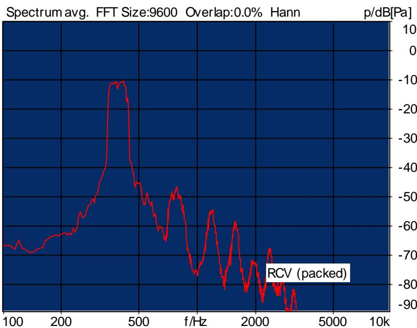
Distortion (Noise) RCV (packed): 33.91 dB (2.02%) Ok
