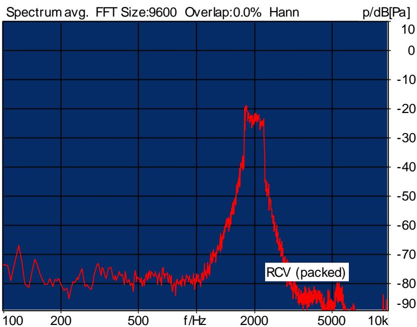
Distortion (Noise) RCV (packed): 21.65 dB (8.27%) Ok
