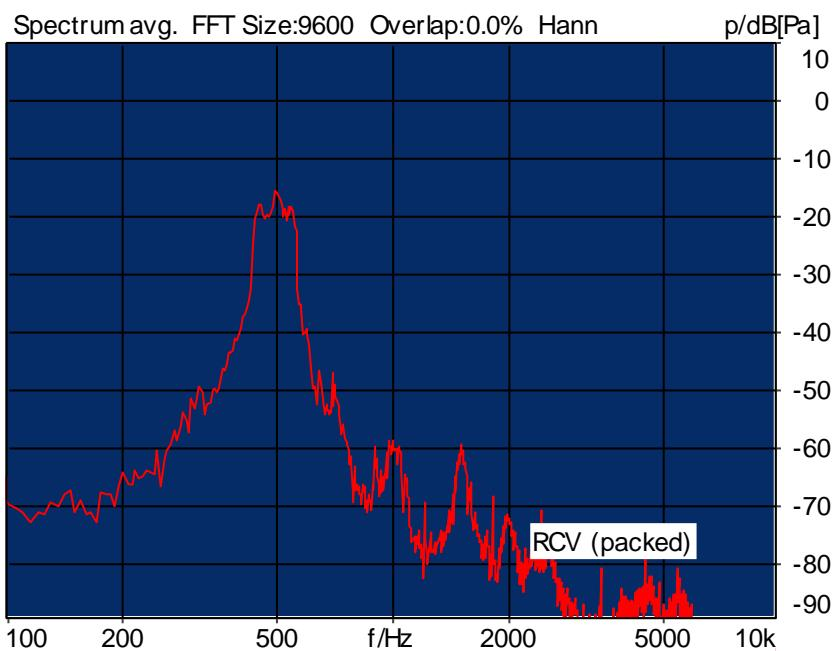
Distortion (Noise) RCV (packed): 28.53 dB (3.74%) Ok
