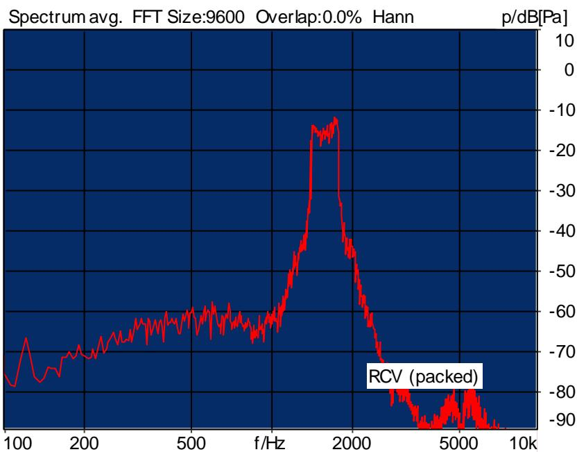
Distortion (Noise) RCV (packed): 26.00 dB (5.01%) Ok
