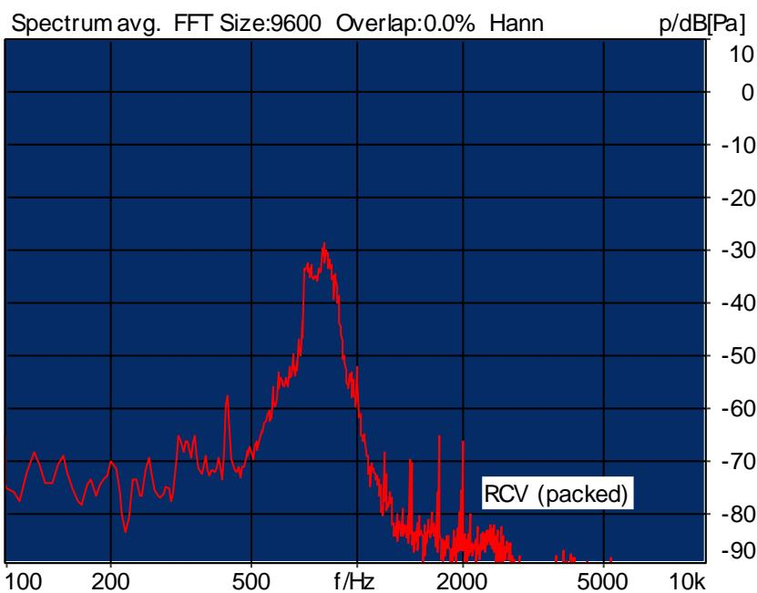
Distortion (Noise) RCV (packed): 22.09 dB (7.86%) Ok
