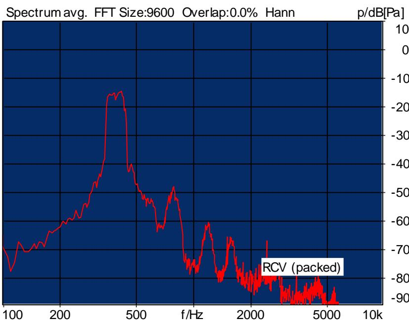
Distortion (Noise) RCV (packed): 31.04 dB (2.81%) Ok
