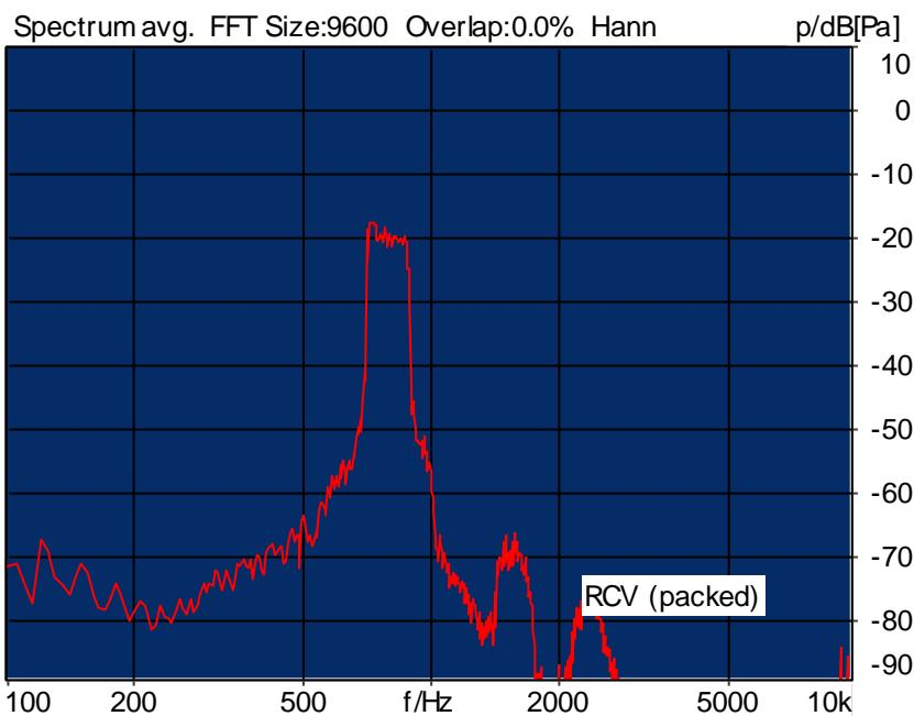
Distortion (Noise) RCV (packed): 35.50 dB (1.68%) Ok
