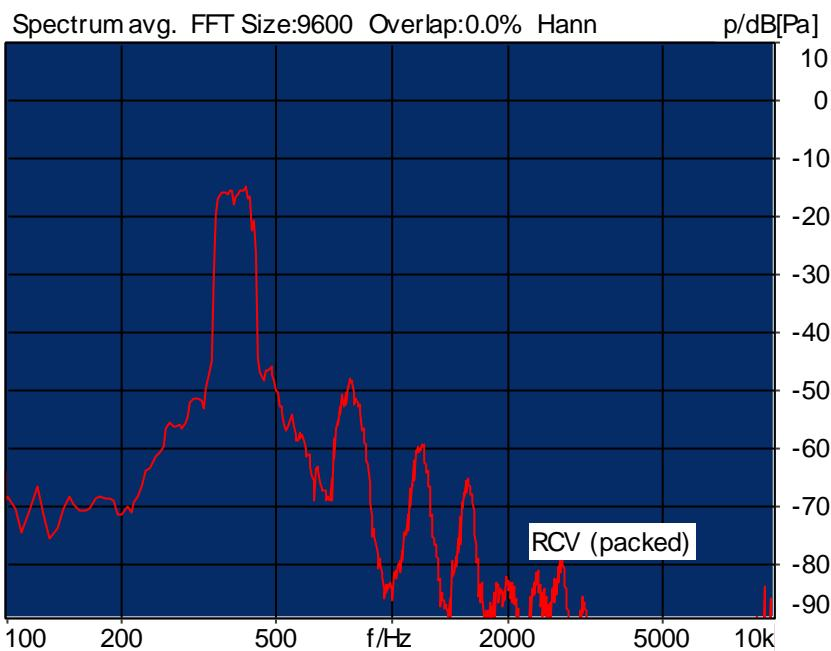
Distortion (Noise) RCV (packed): 32.23 dB (2.45%) Ok
