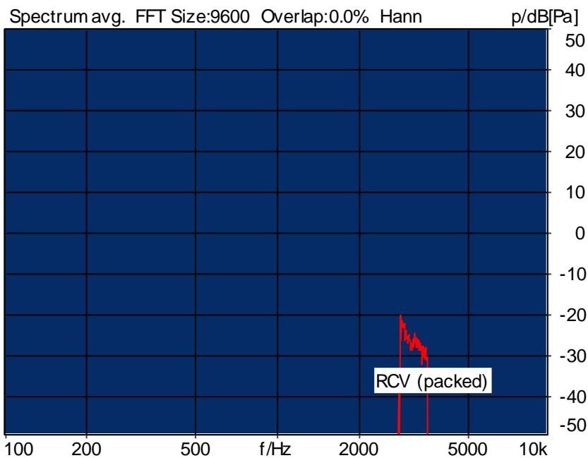
Distortion (Noise) RCV (packed): 40.27 dB (0.97%) Ok
