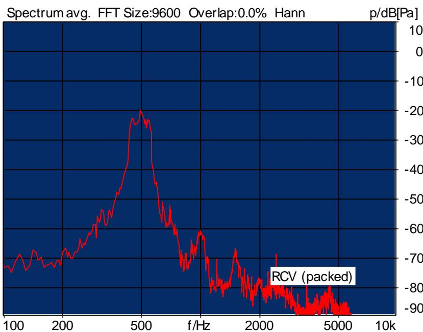
Distortion (Noise) RCV (packed): 28.42 dB (3.79%) Ok
