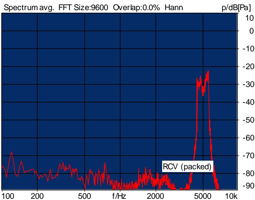
Distortion (Noise) RCV (packed): 32.98 dB (2.24%) Ok
