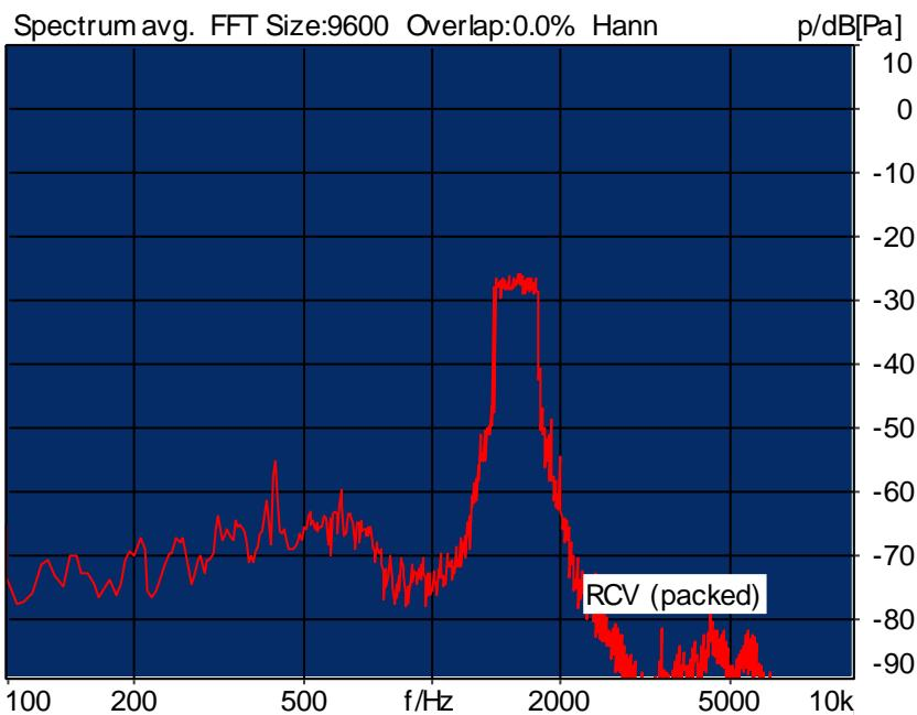
Distortion (Noise) RCV (packed): 26.02 dB (5.00%) Ok
