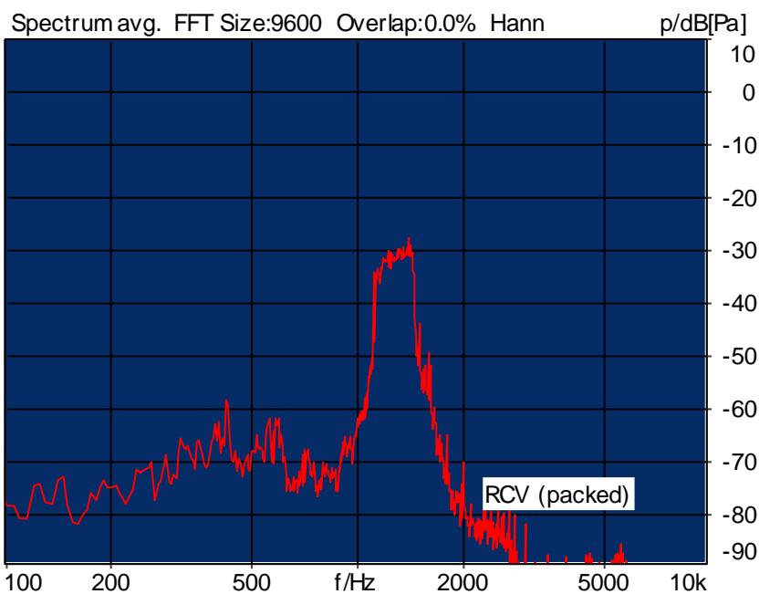
Distortion (Noise) RCV (packed): 20.55 dB (9.39%) Ok
