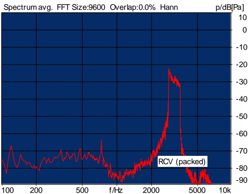
Distortion (Noise) RCV (packed): 29.16 dB (3.48%) Ok
