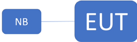
Fig. 2-1 Conducted (Antenna Port) Emission Configuration
