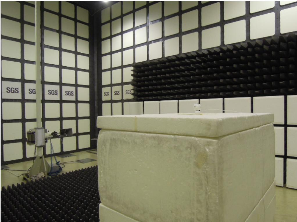
**Radiated Emission Set up Photos (Front View)**
