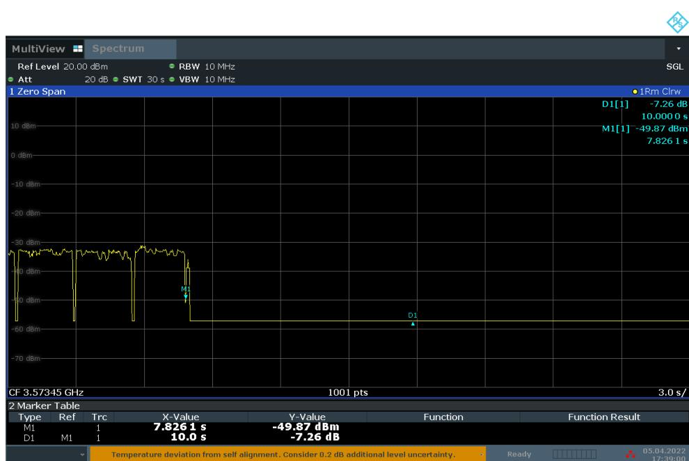
**[Step 5] Setup with 3670-3690MHz & power level 24dBm/MHz****[Step 7] Check EUD Tx Frequency and power**
