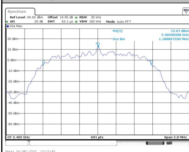
99% Occupied Bandwidth Plot on Channel 00
