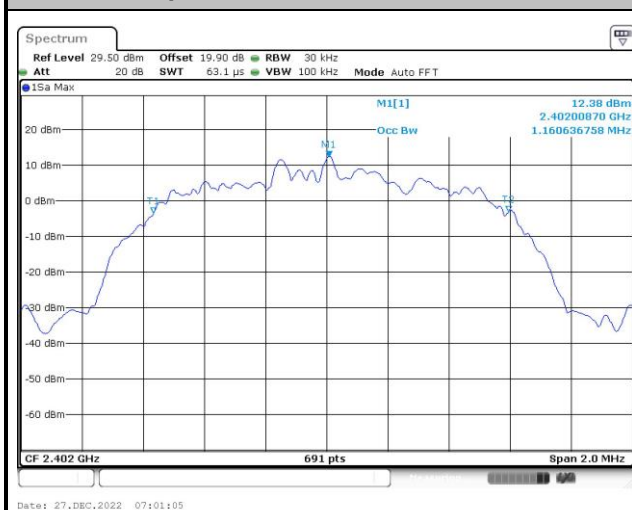
99% Occupied Bandwidth Plot on Channel 00
