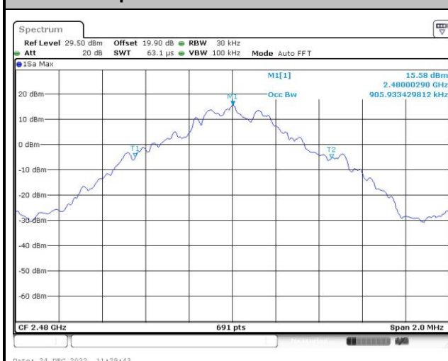
99% Occupied Bandwidth Plot on Channel 78
