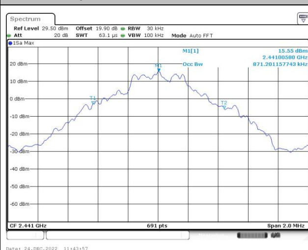
99% Occupied Bandwidth Plot on Channel 39
