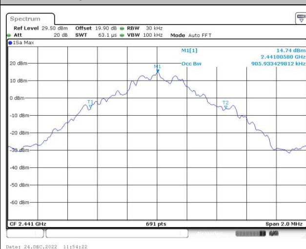
99% Occupied Bandwidth Plot on Channel 39
