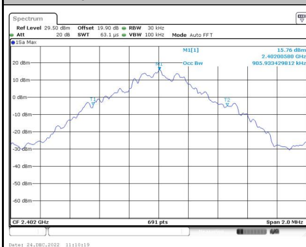
99% Occupied Bandwidth Plot on Channel 00
