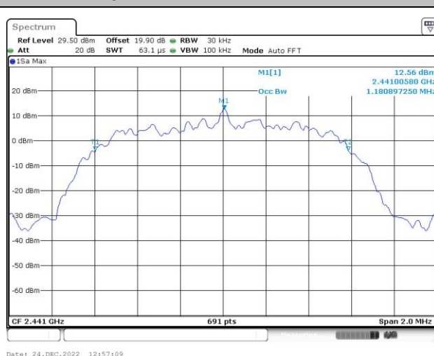
99% Occupied Bandwidth Plot on Channel 39
