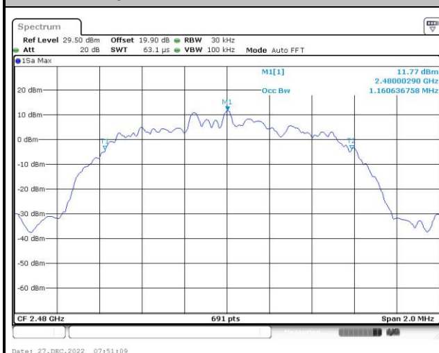
99% Occupied Bandwidth Plot on Channel 78
