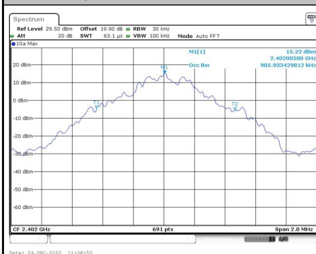
99% Occupied Bandwidth Plot on Channel 00
