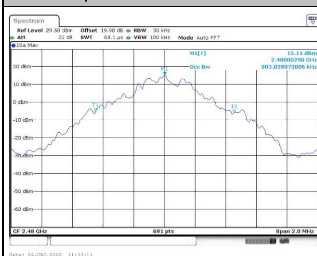
99% Occupied Bandwidth Plot on Channel 78
