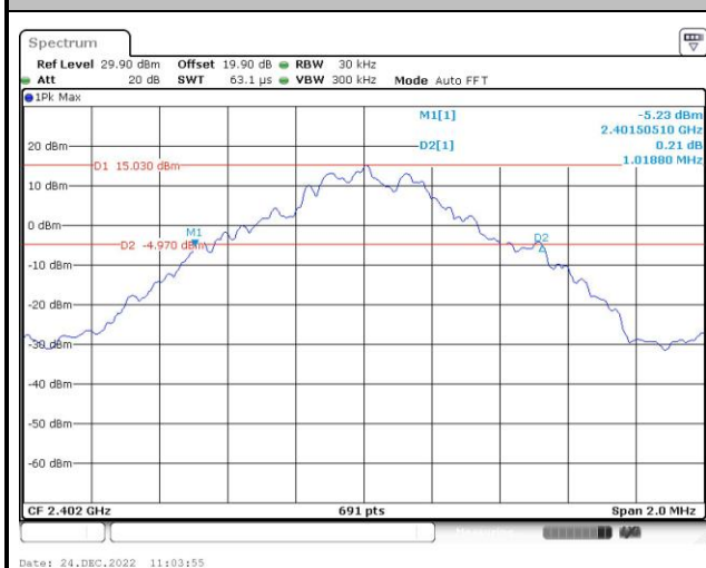
20 dB Bandwidth Plot on Channel 00
