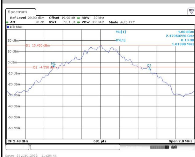
20 dB Bandwidth Plot on Channel 78
