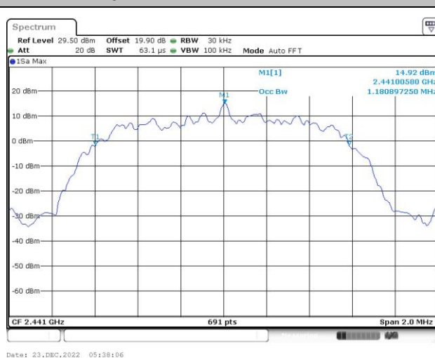
99% Occupied Bandwidth Plot on Channel 39
