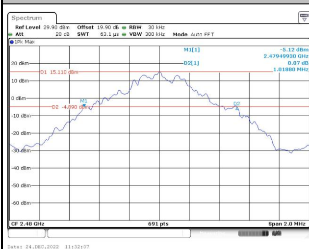
20 dB Bandwidth Plot on Channel 78
