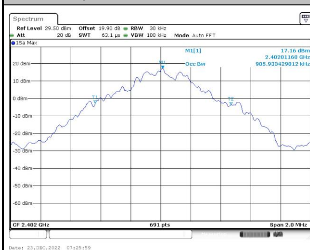
99% Occupied Bandwidth Plot on Channel 00
