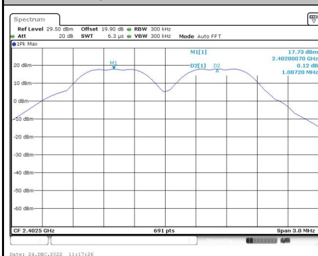
Channel Separation Plot on Channel 00 - 01
