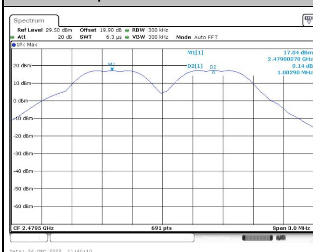
Channel Separation Plot on Channel 77 - 78
