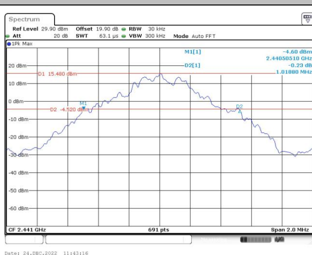
20 dB Bandwidth Plot on Channel 39
