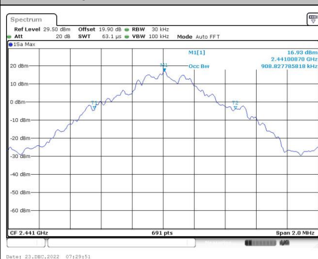
99% Occupied Bandwidth Plot on Channel 39
