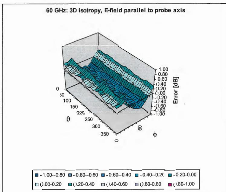
Probe isotropy for  $E_{tot}$ : probe rotated  $\varphi = 0^\circ$  to  $360^\circ$ , tilted from field propagation direction  $\vec{k}$
